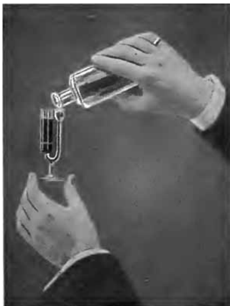
FIG. 22.—Horismascope: adding the reagent.
