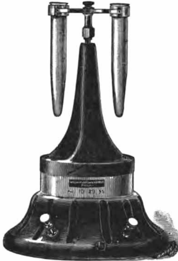
FIG. 16.—The Purdy electric centrifuge.
