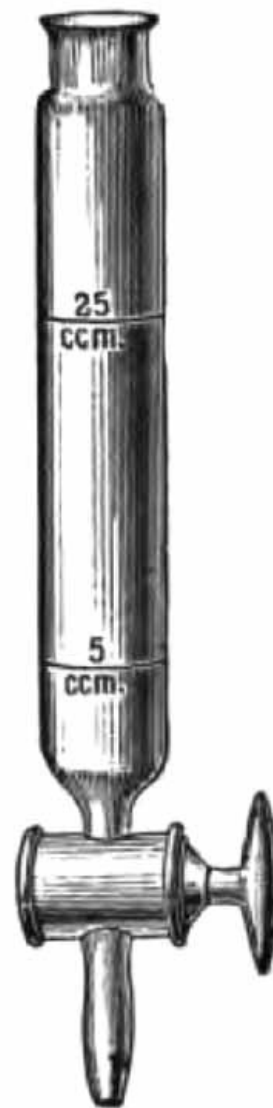
FIG. 87.—Separatory funnel for Strauss' lactic acid test (Sahli).
