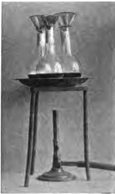
FIG. 28.—"Pancreatic reaction" flasks fitted with funnel condensers on a sand-bath (Robson and Cammidge).
