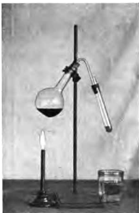
FIG. 26.—A simple distilling apparatus.
