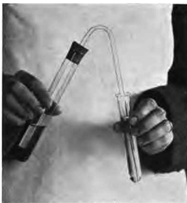
FIG. 30.—A simple hydrogen sulphid generator.
