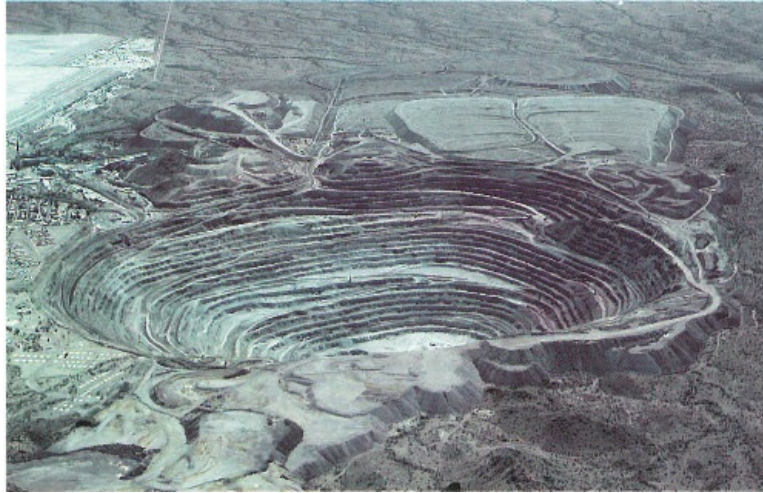
This open-pit mine in the Sonoran Desert near Ajo, Arizona, has exposed an elliptical copper deposit about 1,000 meters long and 750 meters wide. The copper ore mined here is in a bed that averages 150 meters in thickness ( photograph by Peter Kresan ).
