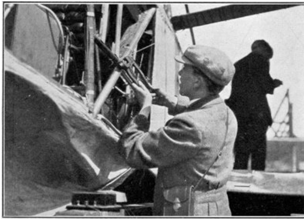
THE LAST TOUCHES—ADJUSTING THE BRACING WIRES
