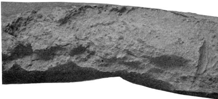
LEAD SERVICE PIPE ILLUSTRATING THE LOCAL EFFECTS OF EIGHT MONTHS' ELECTROLYSIS.
