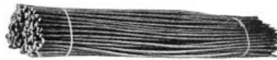
CARTRIDGE OF CORDITE SMOKE-LESS POWDER. Charge for 6-inch 2 F gun, 13 pounds, 4 ounces. Cords, 22 \frac{3}{4} inches long, 3 inches in diameter.
