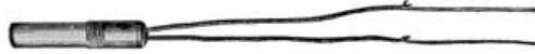
DETONATOR USED IN THE UNITED STATES NAVY. Contains thirty-five grains of fulminate of mercury.
