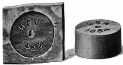
GUN COTTON DISK. With indented inscription, and iron plate upon which the indented inscription has been reproduced.
