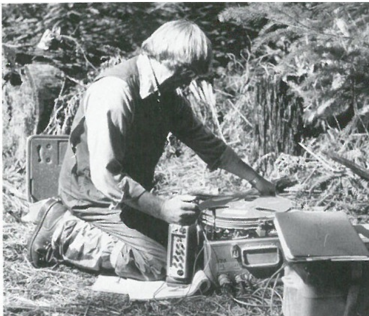
USGS scientist uses portable seismic recording equipment near Mount St. Helens, Washington.
