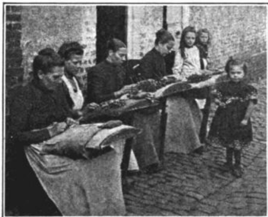
FIG. 59.—Lace being made by hand on pillows with tiny bobbins of thread.
