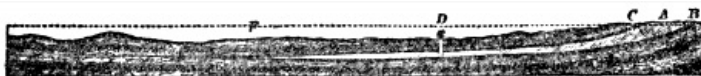
FIG. 21.—Section illustrating the thinning out of a porous water-bearing bed, A, inclosed between impervious beds B and C, thus furnishing the necessary conditions for an artesian fountain at D. (After U. S. Geological Survey.)
