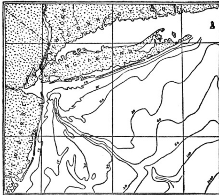
FIG. 1.—The submerged Hudson River channel is clearly shown by the contour lines on the sea floor. Figures indicate depth of water in fathoms. Geologically recent sinking of the land has caused the "drowning" of the river valley. (Coast and Geodetic Survey).
