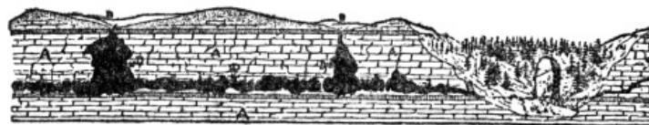
FIG. 23.—Structure section and part of landscape in a limestone region showing how caves and natural bridges are formed by the dissolving action of underground water. AA, limestone; BB, sink holes; DD, caves and galleries; and an arch (natural bridge) which is the remnant of a large cave. (After Shaler, U. S. Geological Survey.)
