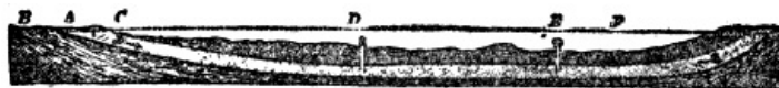
FIG. 20.—Ideal section illustrating the chief requisite conditions of artesian wells. A, a porous stratum; B and C, impervious beds below and above A, acting as confining strata; F, the height of the water level in the porous bed A, or, in other words, the height of the reservoir or fountainhead; D and E, flowing wells springing from the porous water-filled bed A. (After U. S. Geological Survey.)
