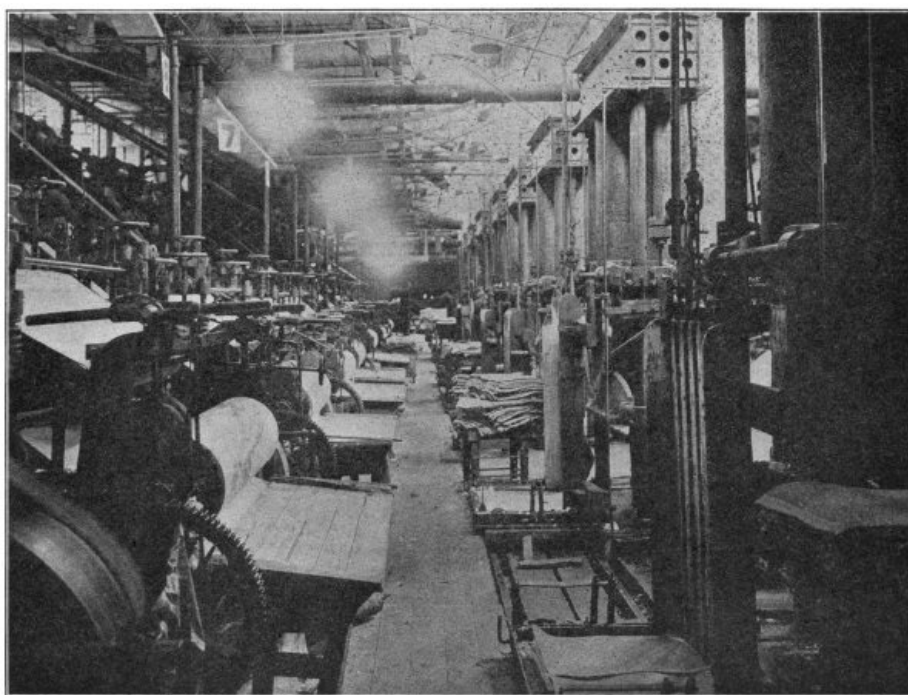
WET MACHINES WHERE THE PULP IS CUT OFF IN SHEETS, THE BROWN CO.
