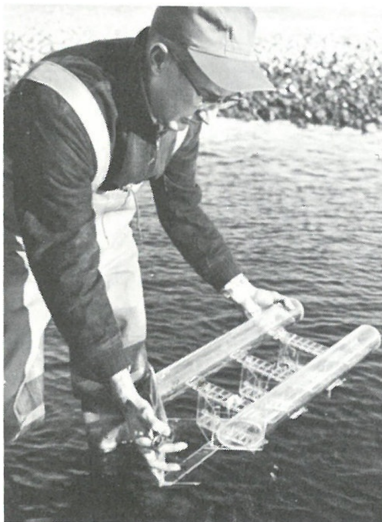
PLANKTON. An ingenious plankton trap is placed in a river as part of a long-range study of radionuclide uptake by aquatic organisms.
