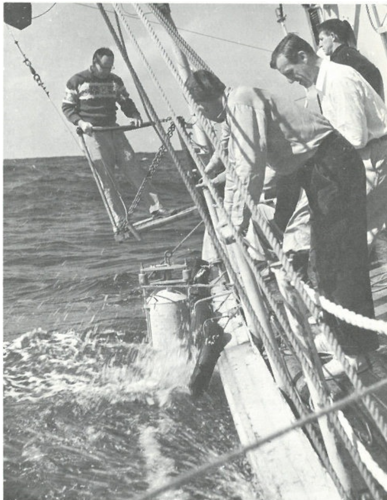
Oceanographers bringing aboard a 50-gallon seawater sampler from the ocean depths find it a difficult task, even in moderate seas. This photo was taken aboard the R. V. Crawford in the Atlantic.
