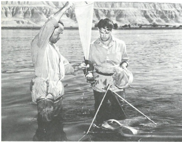
FRESHWATER. Aquatic biologists emptying plankton traps to study concentrations of radioactivity in microscopic organisms in the Columbia River downstream from the Hanford atomic plant in Washington State.
