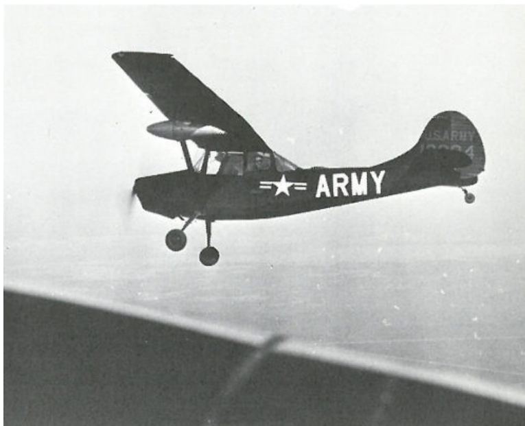
A flying atmospheric physics laboratory studying concentration of radionuclides over an Atomic Energy Commission laboratory. Instrument pod under wing samples air to provide a visual record of radioactivity.
