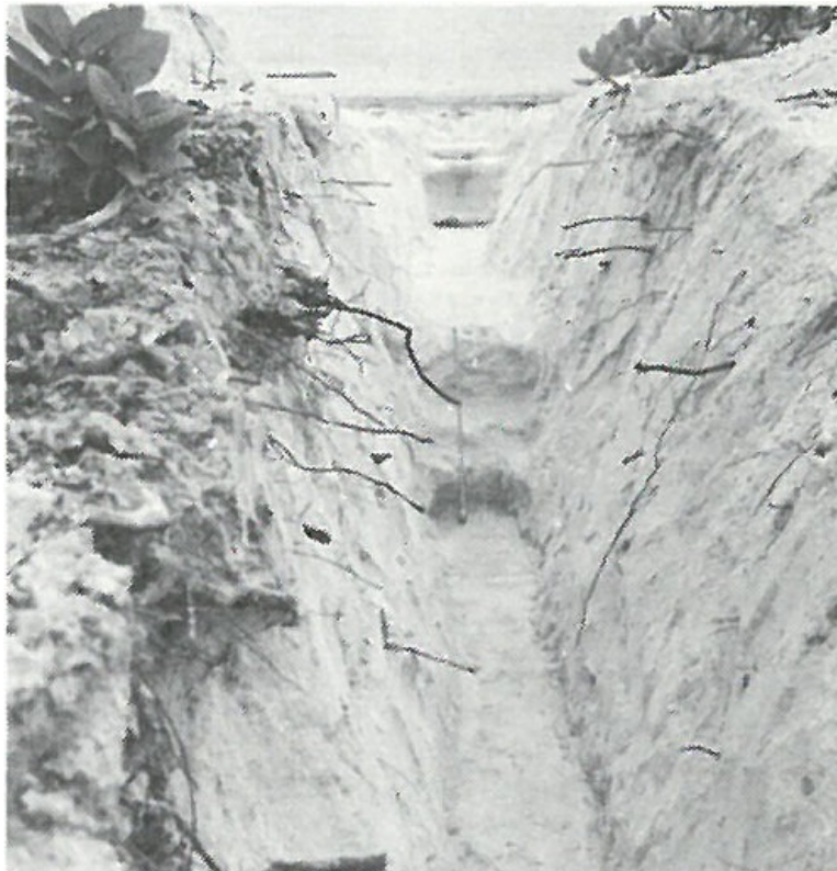
Trench dug on Rongelap Island to expose soil strata and root systems to determine penetration of radionuclides in coral-sand “topsoil”.
