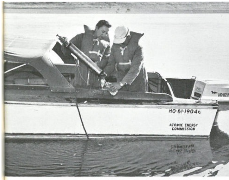
Transferring a sample of water taken from the depths of the Columbia River for radiochemical analysis in a laboratory.
