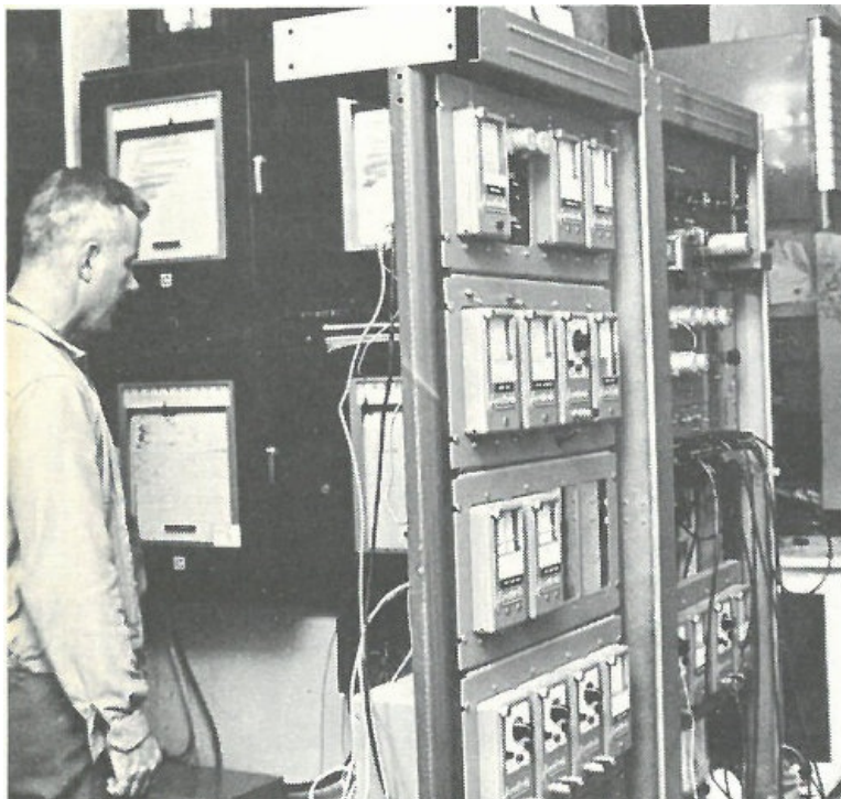
Instruments record radiation, weather, sunlight, and other factors transmitted from remote sensors to this data center established for a long-range terrestrial ecology study program.
