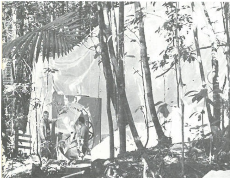
RAIN FOREST. A giant fan pulls air through a plastic-enclosed portion of a Puerto Rico rain forest to study the metabolism rate of trees.
