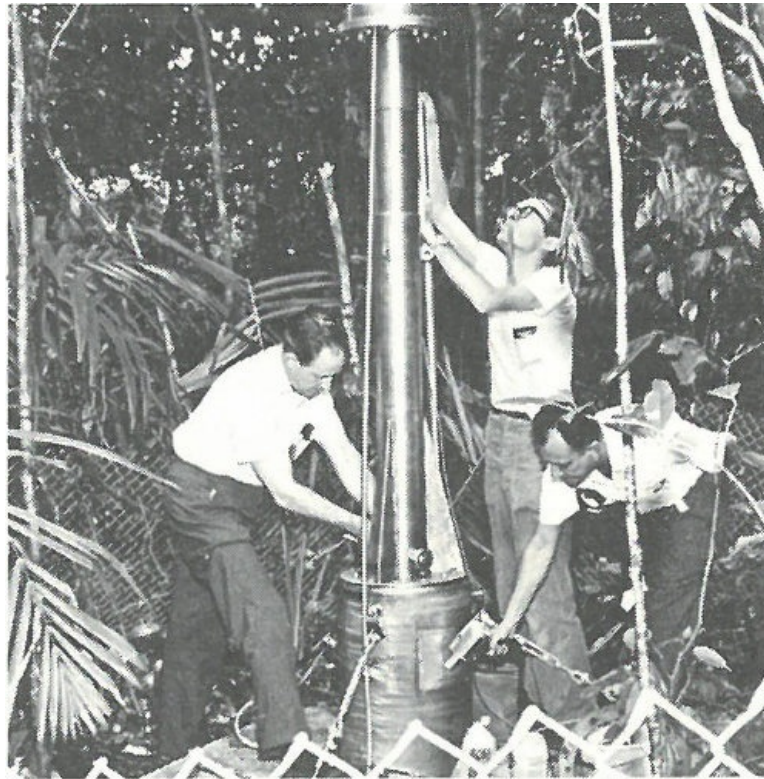
Apparatus containing a strong radiation source being installed by biologists in a semitropical rain forest for terrestrial ecology research.
