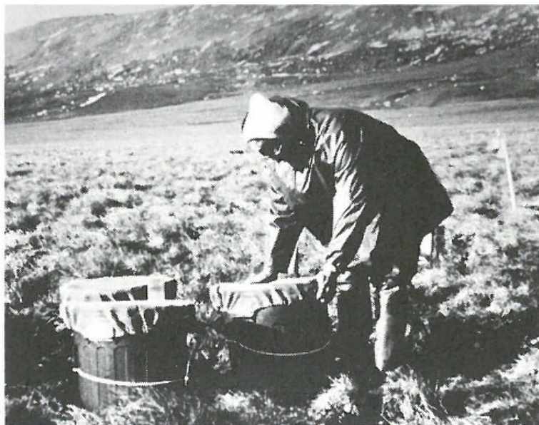
Placing equipment to measure fallout in precipitation north of the Arctic Circle in Alaska.
