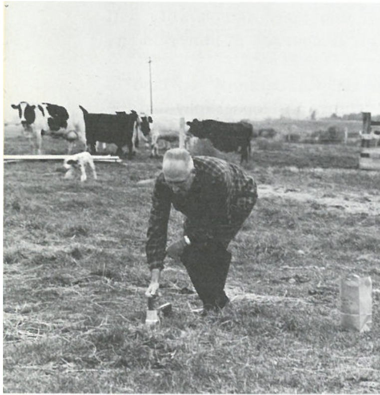
Survey of pasture grasses to determine whether radioactive materials are present. If they are, they could be passed from the grasses to cows and then from the cows' milk to humans.
