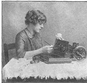
Open and turn back, so that when the oil has soaked through the clogged dirt it may be carefully cleaned away.
