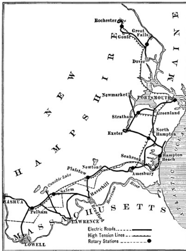
FIG. 52.—Transmission Line of New Hampshire Traction Company.
