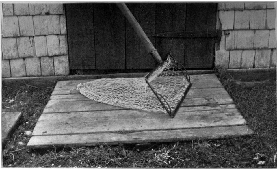
The Scallop Pusher. —This implement consists of a wooden pole, from 8 to 9 feet long, attached to a rectangular iron framework, 3 by 1½ feet, fitted with a netting bag, 3 feet in depth. The scalloper, wading in the shallow water, gathers the scallops from the flats by shoving the pusher among the eel grass. The photograph shows the correct position of the pusher in operation. Only a small part of the pole is shown.
