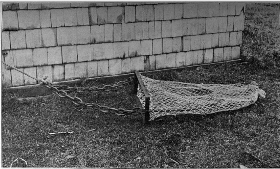
The Box Scallop Dredge. —This dredge consists of a rectangular framework, 27 by 12 inches, with an oval-shaped iron bar extending backward as a support for the netting bag, which is attached to the rectangular frame. To the sides of this frame is joined a heavy iron chain about 4 feet long, to which the drag rope is fastened. This style of dredge is used only at Chatham and the neighboring towns of Cape Cod.
