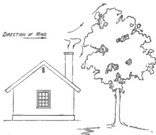
Fig. 4.—Large trees located near chimney tops may deflect wind currents down the chimney. This may be avoided by placing the chimney on the opposite side of the building.
