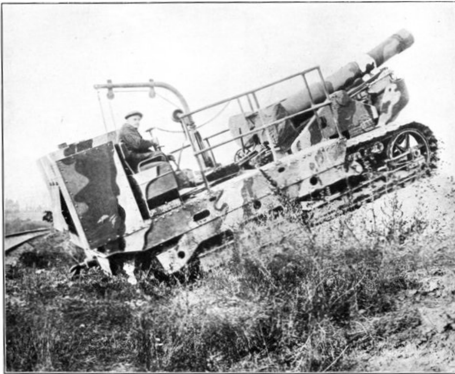
CATERPILLAR TRACTOR MOUNTING AN 8-INCH HOWITZER WHICH HAS A RANGE OF 6 MILES WITH A PROJECTILE WEIGHING 200 POUNDS.
