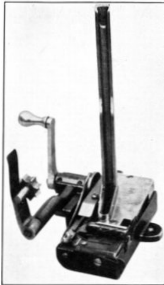
BELT-FILLING MACHINE FOR BROWNING MACHINE GUN, MODEL 1917.
