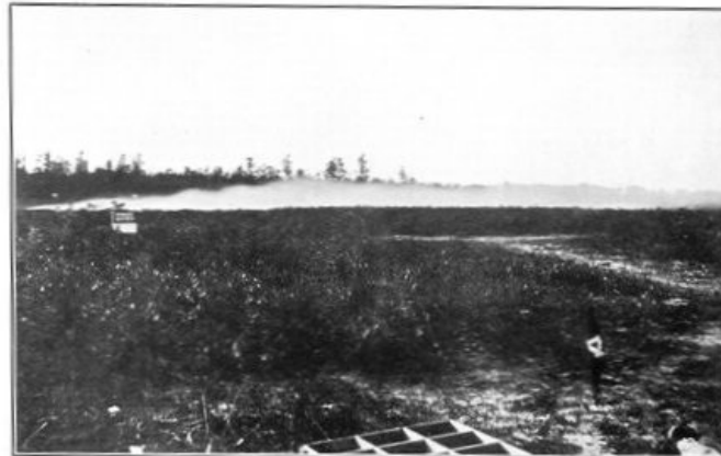
GAS CLOUD FROM 4.7-INCH GAS SHELL EXPLODING 8,533 YARDS FROM THE GUN AT LAKEHURST.
