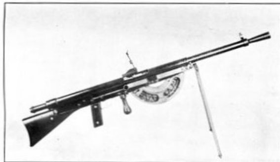
CHAUCHAT MACHINE RIFLE, MODEL 1915, CALIBER, 8 MILLIMETERS.
