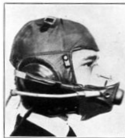
AVIATOR'S OXYGEN HELMET EQUIPPED WITH TELEPHONE RECEIVER.
