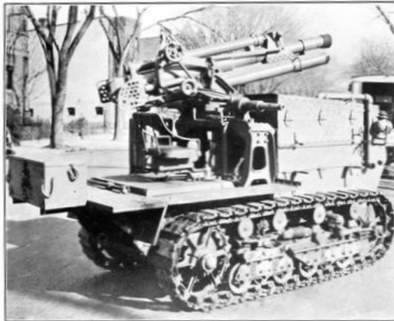
CATERPILLAR TRACTOR WITH 3-INCH GUN MOUNTED ON IT.
