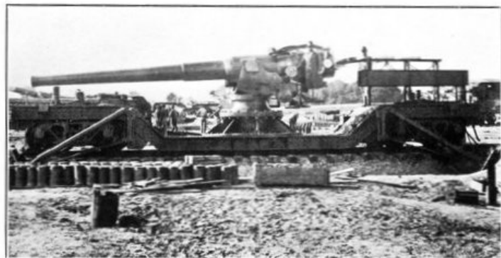
TWO VIEWS OF THE 7-INCH NAVY RIFLE MOUNTED ON A PEDESTAL ON A RAILWAY CAR.
