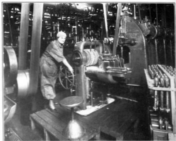
MACHINING THE CONNECTING RODS FOR THE LIBERTY ENGINE. CADILLAC MOTOR CO.
