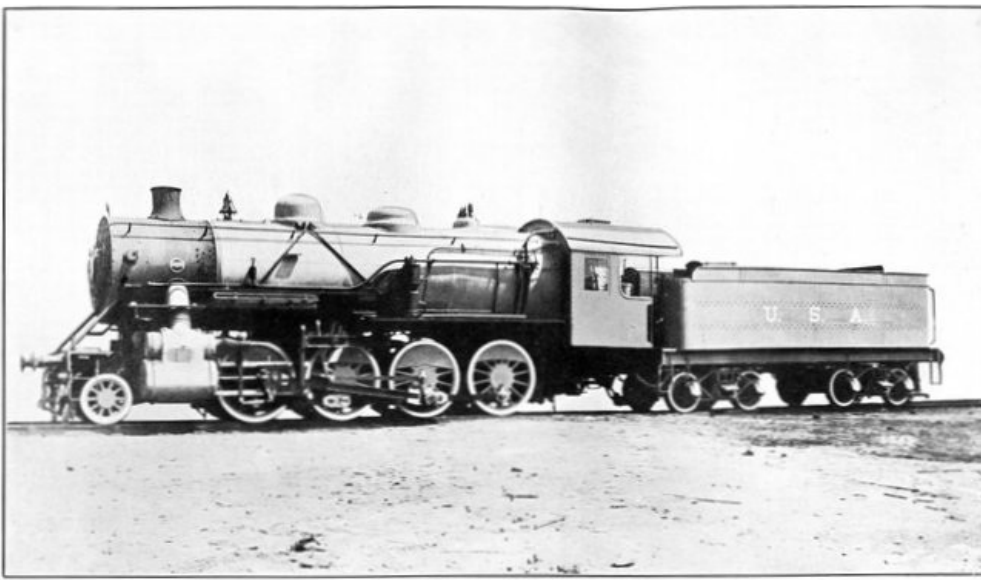
STANDARD GAUGE 10-WHEEL CONSOLIDATION (BALDWIN) LOCOMOTIVE. CYLINDER, 21 INCHES × 28 INCHES.
