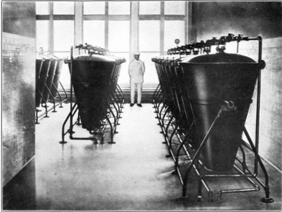
MANUFACTURING BARRINGTON-HALL SOLUBLE COFFEE AT THE BAKER IMPORTING CO. PLANT, NEW YORK. THREE BATTERIES OF 21 PERCOLATORS. CAPACITY 5 CASES OF COFFEE EACH.
