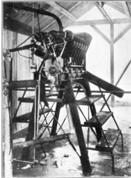
TEST SHED AND STAND WITH LIBERTY ENGINE MOUNTED WITH TEST PROPELLER. PACKARD MOTOR CAR CO.
