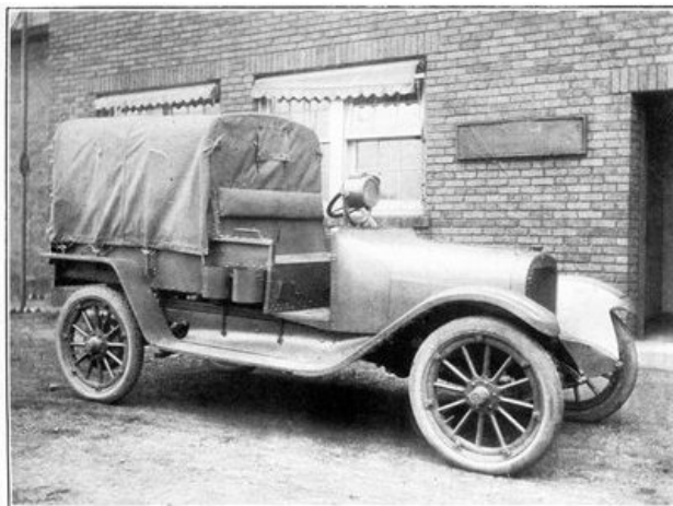
LIGHT REPAIR TRUCK ON DODGE CHASSIS. Special body with tools for making minor motor repairs.
