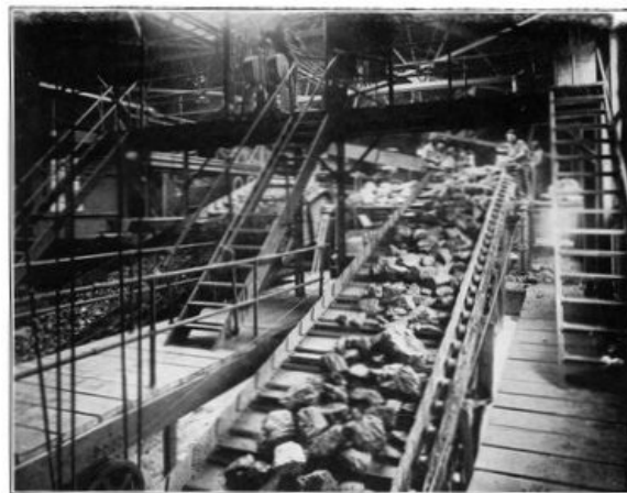
PICKING TABLES AND LOADING BOOMS IN A WEST VIRGINIA COAL MINE.
