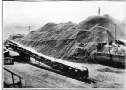
1,200 TONS OF APRICOT PITS AT SAN FRANCISCO READY TO BE REDUCED TO CARBON FOR GAS MASKS.
