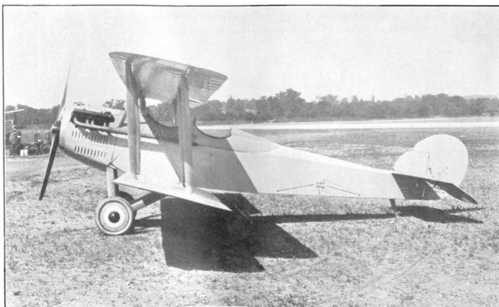
V. E. 7. EQUIPPED WITH 180-HORSEPOWER HISPANO-SUIZA ENGINE.
