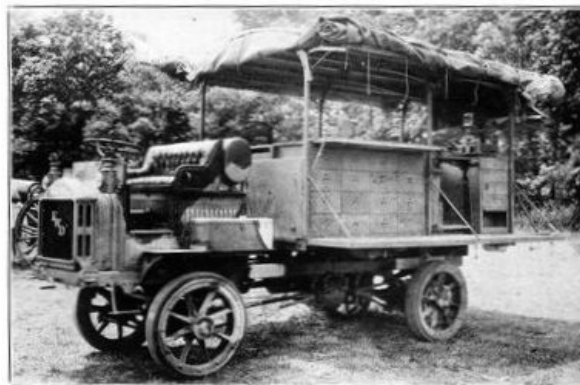
ORDNANCE EQUIPMENT REPAIR TRUCK ON F. W. D. CHASSIS.
