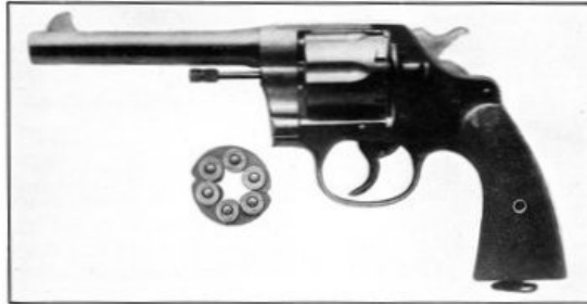
COLT DOUBLE ACTION REVOLVER, CALIBER .45, MODEL 1917.
