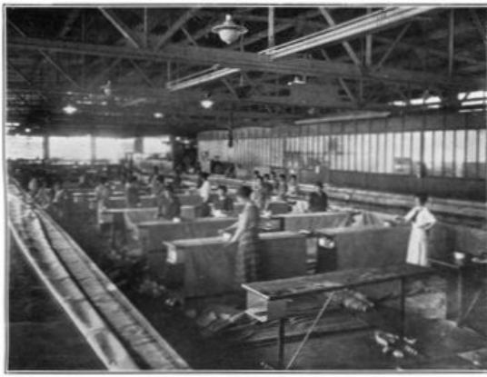
CUTTING AND CEMENTING BALLOON PANELS IN THE GOODRICH PLANT AT AKRON.
