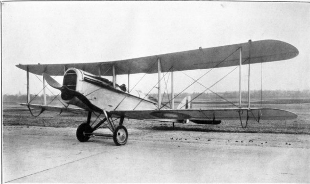
DE HAVILAND-4. USED FOR OBSERVATION, RECONNAISSANCE, COMBAT, DAY BOMBING, AND DEFENSIVE FIGHTING.
