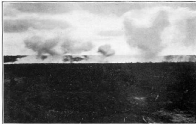
PHOSPHORUS CLOUDS FROM BURSTS OF 75- MILLIMETER SHELL AT LAKEHURST, N. J., PROVING GROUNDS.
