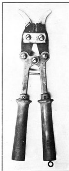
WIRE CUTTER, MODEL 1918, SHOWING SPECIAL RUBBER HANDLES.
