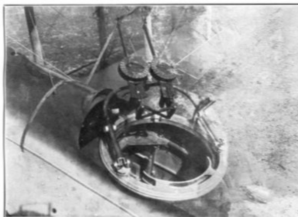
TWO LEWIS MACHINE GUNS WITH MOVABLE MOUNTING, IN THE OBSERVER'S COCKPIT OF A DE HAVILAND-4.
