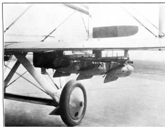
TWO VIEWS, MARK V RELEASE TRAP (RIGHT HAND) WITH UNIVERSAL NOSE AND TAIL BEAM, MOUNTED ON T-RAILS UNDER RIGHT WING OF DH-4 PLANE.
