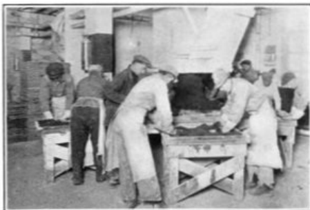
Slabbing the doughlike mixture of carbon and spreading it on screen-bottomed trays at carbon plant No. 2.
