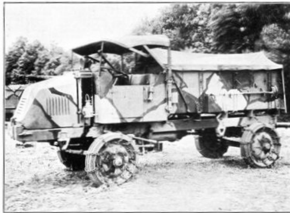
AMMUNITION TRUCK MOUNTED ON STANDARD ORDNANCE FOUR WHEEL DRIVE TRACTOR.
