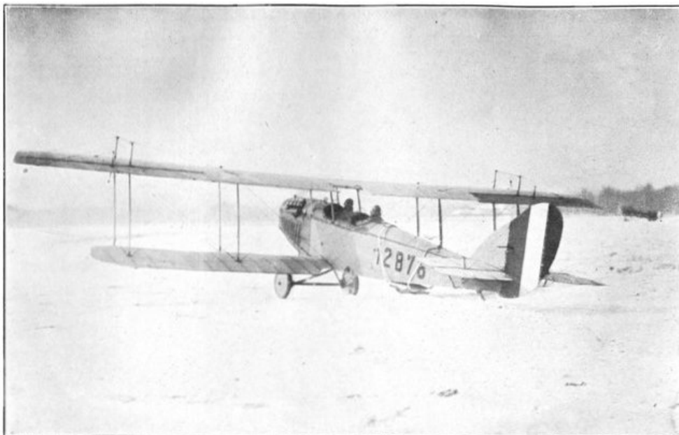
CURTISS JN4-D, USED AS A PRIMARY TRAINING MACHINE. ENGINE, CURTISS OX-5.
