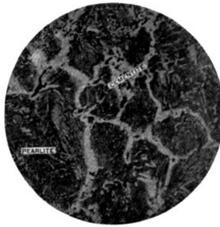
Steel containing more than nine-tenths of one per cent of crystals of pearlite, surrounded by envelopes of cementite ( Fe_3C ). Magnified 200 diameters.
