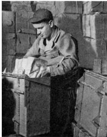
Figure 42: Leaflet Distribution: Packing the Boxes. Sometimes boxes were used instead of bombs. These, being square, facilitated the packing process, since the rectangular packages could be used just as they came out of the printshop. The fuze is attached to the package, not to the box.
