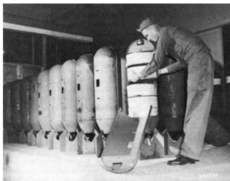
Figure 76: Korean Leaflet Bomb, Early Model. An M16A1 cluster adapter being loaded at the FEC printing plant in Yokohama (1 November 1950). The bomb type adapter will contain 22,500 (5" by 8") psychological warfare leaflets.
