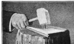
Driving a nail with a hammer made of mercury frozen by Liquid Air.
