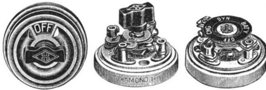
FIGS. 464 and 465.—Snap switch; views showing switch with cover on, and exposed to show mechanism. The switch is provided with indicating dial which registers "on" and "off" positions.
