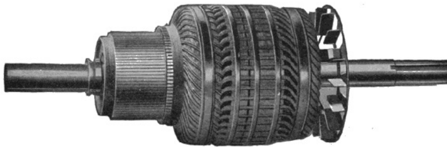
FIG. 366.—Western Electric barrel wound armature, having a fan attached at one end to induce a circulation of air for ventilation.
