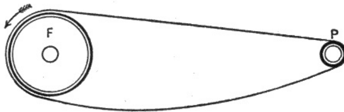
FIG. 447.—Wrong way to run a belt. The pull should not come on the top side, because, with slack at bottom there is a tendency to slip.
