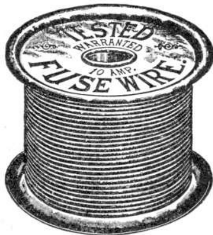
FIG. 467.—Spool of fuse wire. The wire is usually made of an alloy of tin and lead, such as half and half solder. Bismuth is frequently added to the alloy to lower the melting point. For half and half solder the melting point is 370° Fahr. The quickness with which a fuse will melt after the current has reached the limit depends upon the specific heat and latent heat of the metal. The current required to "blow" a fuse increases somewhat with the age of the fuse owing to oxidation and molecular changes. Fuses are sometimes rated according to the number of amperes to be taken normally by the circuit they are to protect. Thus, a 10 ampere fuse is supposed to protect a circuit whose regular current should not exceed 10 amperes, and to blow if the current rise to say 12 amperes. The Underwriters' rule requires that the rating be about 80% of the maximum current it can carry indefinitely, thus allowing about 25% overload before the fuse melts. The fusing current varies considerably according to circumstances. The temperature of the surrounding air or other substances affects the melting current greatly, because the rate at which heat from the fuse will be transferred to the surroundings depends upon the difference of temperature between them and the fuse. Hence a fuse in a warm place will be melted by a smaller current than a similar fuse in a cold place. For a similar reason, a fuse in an enclosed place where there is little chance for the heat to be dissipated, will melt with a smaller current than the same in an open place. If the current increase gradually to that which would ordinarily melt the fuse, the high temperature makes the fuse wire oxidize rapidly; this sometimes makes a sort of tube of oxide which will not break even after the fuse wire inside has melted, and so the fuse carries more than its rated current. Open fuses are so unreliable that circuit breakers are preferable for large currents; when fuses are used, the enclosed type as shown in figs. 468 to 470, is usually the more desirable.
