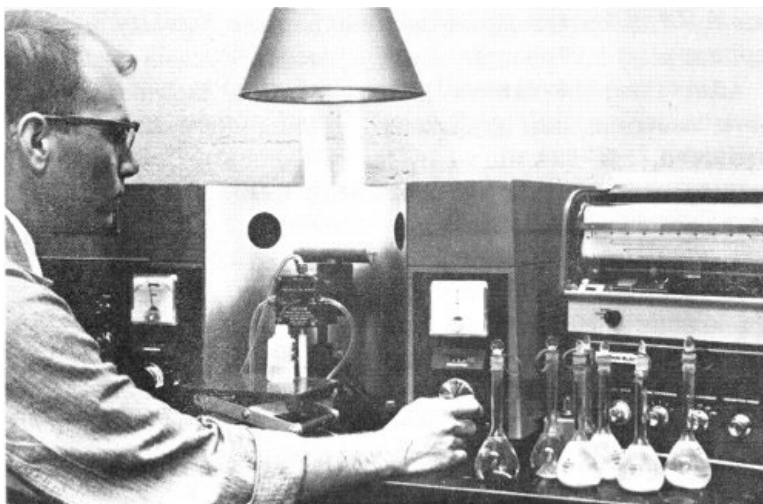
An atomic absorption spectrophotometer is used to measure the amount of potassium in samples of mica dissolved in acid.
