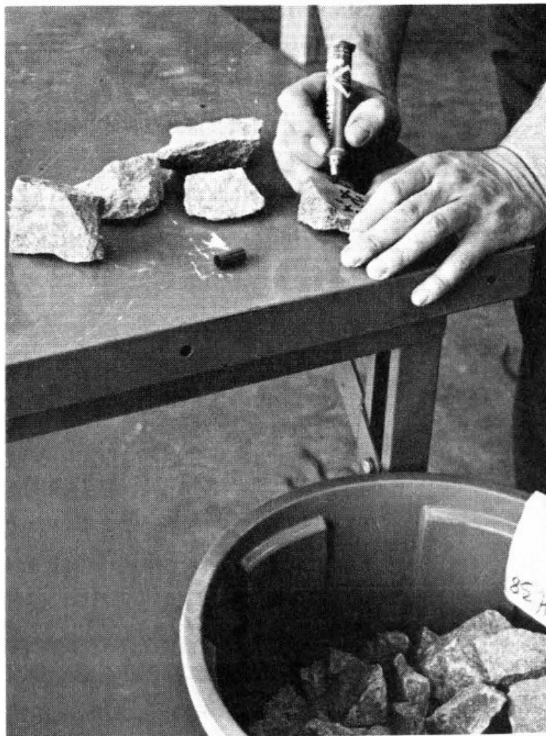
A sample of granite being made ready for crushing and mineral separation.
