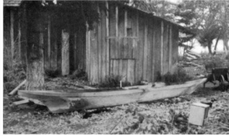
THE FINISHED HULL OF THE CANOE SHOWN IN PLATES IV AND V To the left in the photograph is the bow, which in this case lacks the "notch" found in many specimens. The "lift" of the boat's lines toward the prow may be plainly seen. This enables it to ride the waves. (Photograph by J. D. Leechman.)
