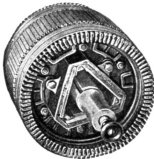
FIG. 1,764.—Western Electric wound armature for internal resistance induction motor. In starting the inductors are short circuited through a resistance which is gradually cut out as the motor comes up to speed.
