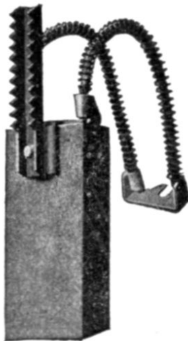
FIG. 2,055.—Detail of Westinghouse commutating pole rotary converter brush, showing rack. The brush lifting mechanism and its operation is explained in fig. 2,050.
