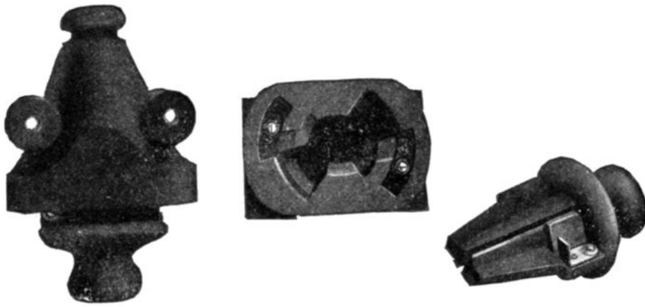
FIGS. 1,961 TO 1,963.—Fuse blocks for Westinghouse transformers. The fuses furnished with the transformers are mounted in a weather proof porcelain fuse box of special design. The stationary contacts are deeply recessed in the porcelain and are well separated from each other. The contacts are so constructed that the plug is held securely in place by giving it a partial turn after inserting it. When the plug is in position, the fuse is in sight and its condition can be noted which eliminates all danger of pulling the fuse while same is still intact and the transformer is under load.
