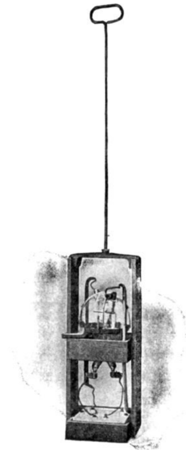
FIG. 2,100.—Westinghouse-Cooper Hewitt mercury vapor rectifier bulb and box. The life of the bulb is materially increased by operating it at certain temperatures and for this reason the bulbs in the arc light rectifier outfits are immersed in oil and mounted in the same tank with the regulating transformer. Two bulbs in series are used with the 75 light outfit. The bulb is mounted on tilting trunnions in a box
