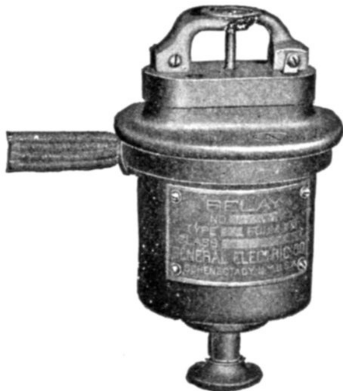
FIG. 2,301.—Alternating current low voltage circuit closing low voltage relay, for 600 volts or less. The contacts are similar to those of the circuit closing overload type except that they are inverted. As long as the pressure is normal the contact cone is held above the contacts. When the pressure falls below one half normal, the cone and plunger rod drop and close the contact. This relay does not pick up its own plunger. The plunger rod is pushed up by hand after the pressure circuit is
