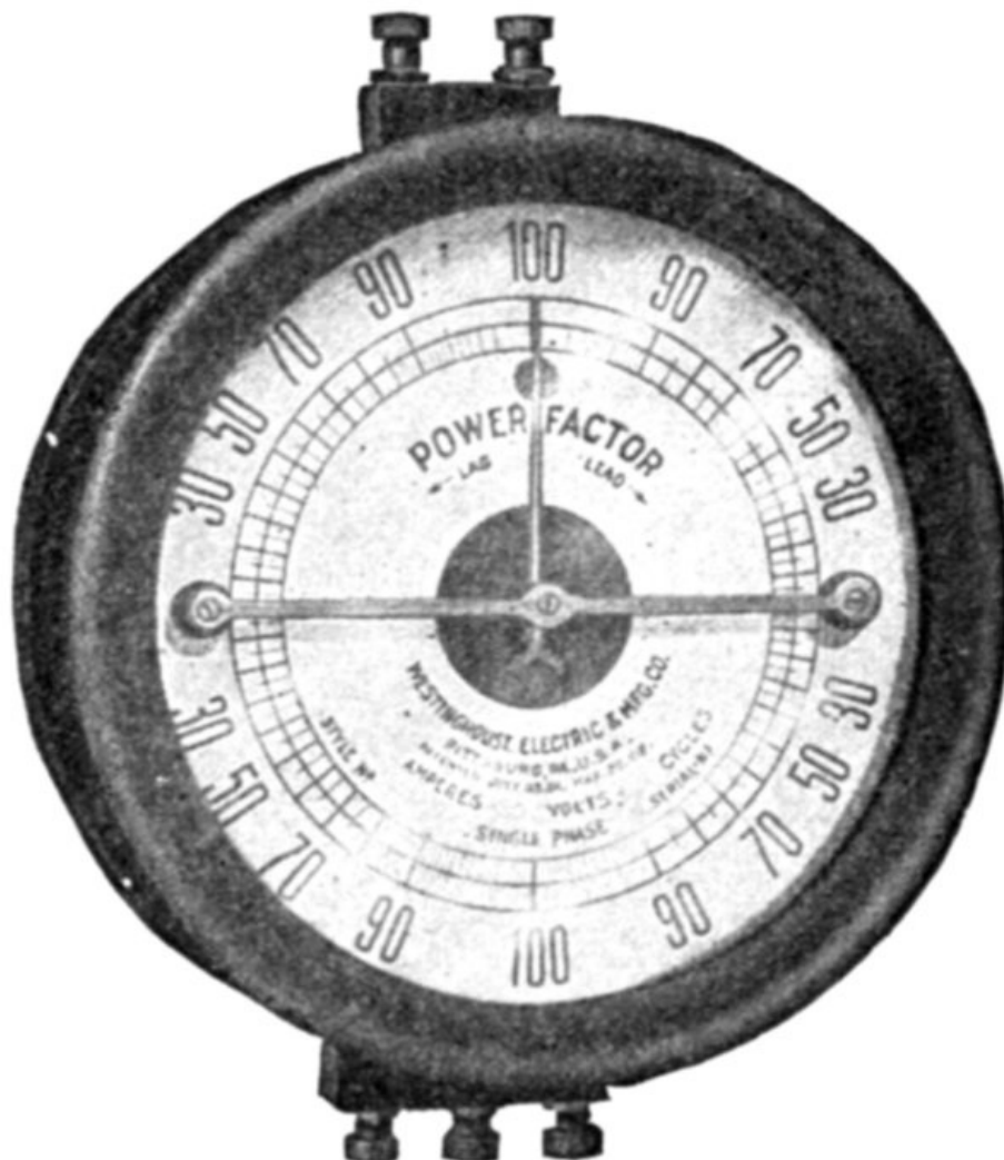
FIG. 2,578.—Westinghouse rotating field type power factor meter. The rotating field is produced by the currents of the metered circuits in angularly placed coils, one for each phase of the system, in the case of polyphase meters. In the three phase meter the rotating field is produced by three coils spaced 60° apart; in the two phase meter by two coils spaced 90°; in the single phase meter the positions of voltage and current coils are interchanged and the rotating field is produced by means of a split phase winding, connected to the voltage circuit. There are no movable coils or flexible connections. Single phase meters indicate the power factor of a single phase circuit, or of one branch of any polyphase circuit. Special calibration is necessary in order to use a single phase instrument on a three phase circuit unless the voltage coil be connected from one line to the neutral. Polyphase meters
