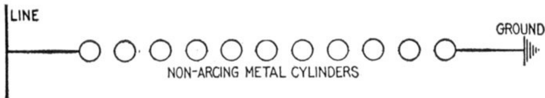
FIG. 2,349.—Non-arcing multi-gap arrester. Based on the principle of employing for the terminals across which the arc is formed, such metals as are least capable of maintaining an alternating arc between them. This so called non-arcing property of certain metals was discovered by Alexander Wurtz. The action is such that the "line current" which follows the lightning discharge follows as an arc, but is stopped at the end of one alternation because of the property of the non-arcing metals to carry an arc in one direction, but requiring an extremely high voltage to start a reverse arc. The non-arcing metals ordinarily employed are alloys of zinc and copper. Plain multi-gap arresters as here shown operate satisfactorily with the smaller machines and on circuits of limited power, but for large machines of close regulation, and therefore of very large momentary overload capacity, especially when a number of such are operated in parallel, such arresters were found insufficient, the line current following the lightning discharge frequently was so enormous that the circuit did not open at the end of the half wave, that is the arrester held the arc and was destroyed. The introduction of synchronous motors made it necessary that the arc should be extinguished immediately, otherwise the synchronous motors and converters would drop out of step, and the system would in this way be shut down. To insure the breaking of the arc, resistance was introduced in the arrester, the modified device being known as the low equivalent arrester as shown in fig. 2,350.
