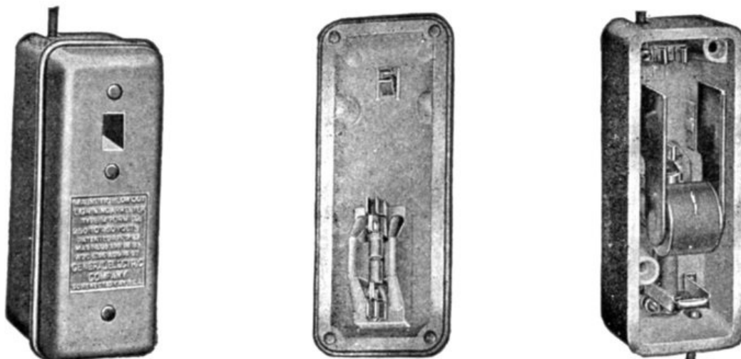
FIGS. 2,402 to 2,404.—General Electric magnetic blow out arrester for use on railways. It consists of an adjustable spark gap in series with a resistance. Part of the resistance is in shunt with a blow out coil, between the poles of which is the spark gap. The parts are mounted in a strong, porcelain box, which, for car and pole use, is in turn mounted in a substantial asbestos lined, wooden box. In operation, when the lightning pressure comes on the line, it causes the spark gap to break down and a discharge occurs through the gap and the resistance rod to ground. Part of the current shunts through the blow out coil producing a strong magnetic field across the spark gap. The magnetic field blows out the discharge arc and restores normal conditions. The resistance is only 60 ohms (for 500 volt rating work), and the spark gap only one-fortieth of an inch (.025 in.).
