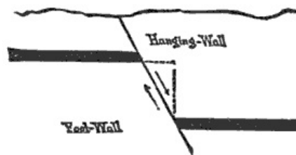
Fig. 28.—Section of a normal fault.
