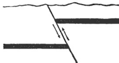
Fig. 29.—Section of a reversed fault.
