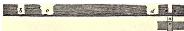
Fig. 238.—Beam, or Stretcher, binding tops of Piles, 10 ft. 6 in. long by 9 in. broad.
