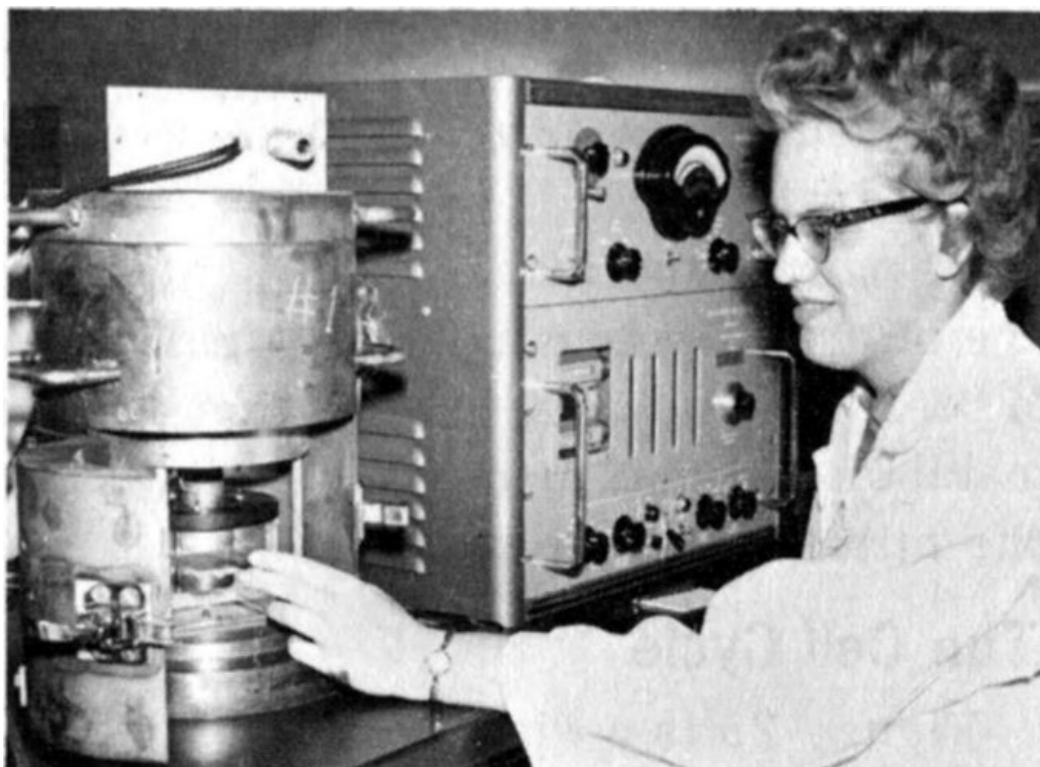
Figure 24 A college chemistry major analyzing a sample of radioactive materials with an instrument known as a proportional beta counter.
