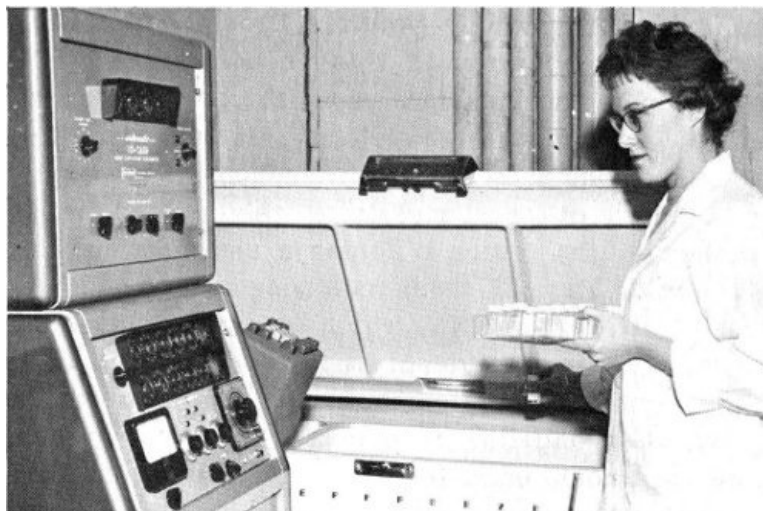
Figure 19 Placing radioactive samples in a refrigerated unit for liquid scintillation counting.
