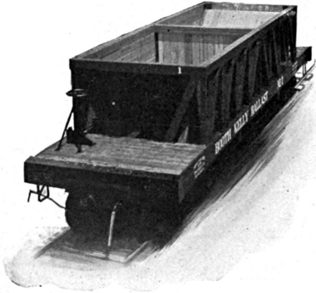
View of Standard Ballast Car, showing arrangement of Hoppers
