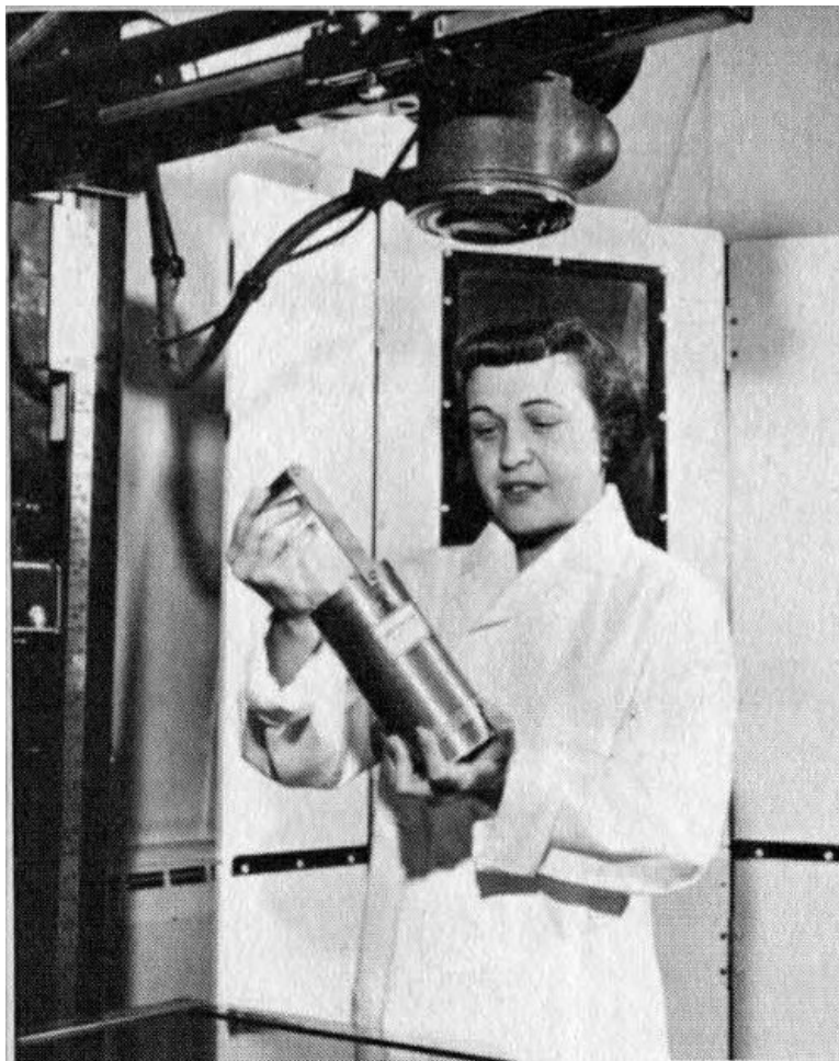
A technician holds an inexpensive portable X-ray unit that was developed by the Argonne National Laboratory. Compare its size with the standard X-ray machine shown at left and above.
