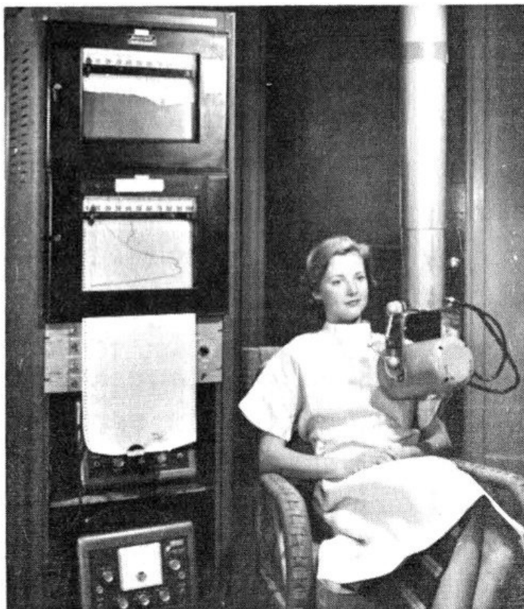
In this cardiac output study a probe is positioned over the heart and the passage of iodine-131 labeled human serum albumin through this area is recorded.
