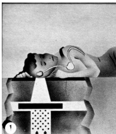
(1) A lead shutter shields the patient from reactor neutrons.
