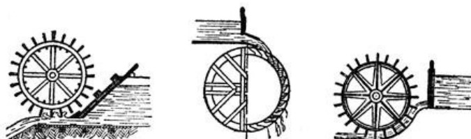
FIG. 30.—UNDERSHOT, OVERSHOT, AND BREAST WHEELS
