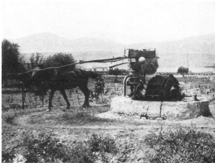
A HORSE-OPERATED CHAIN-PUMP USED IN GREECE
