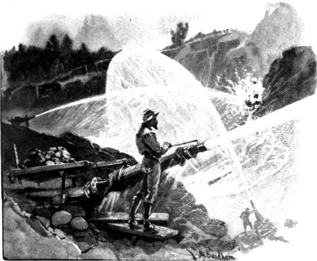
"MONITORS" AT WORK—THE PRESSURE OF THE WATER IS SO TERRIFIC THAT THE SOLID ROCK IS LITERALLY WASHED AWAY. OUR ILLUSTRATION IS FROM A DRAWING MADE BY MR. SANDHAM WHILE IN CALIFORNIA.
