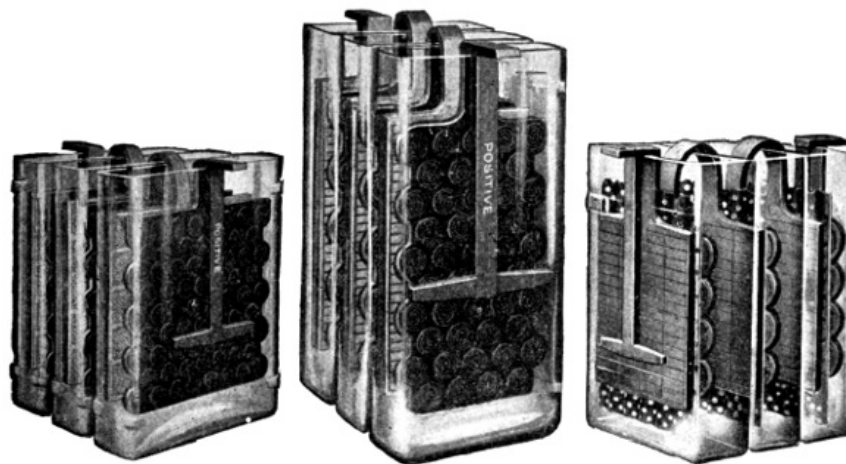
FIGS. 1,124 to 1,126.—Electric Storage Battery Co. chloride cells. The voltage of cells of all capacities is slightly above 2 volts on open circuit, and during discharge at the 8 hour rate it varies from that point at the beginning to 1.75 volts at the end.
