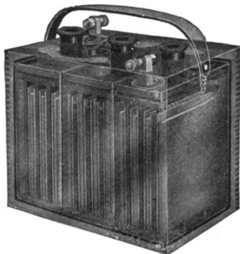
FIG. 1,091.—Phantom view of an "Exide" sparking or ignition battery. It contains three cells. In this type, the terminal lug has been designed to obviate the creeping of the electrolyte with its accompanying corrosion. The positive and negative terminals are for identification.
