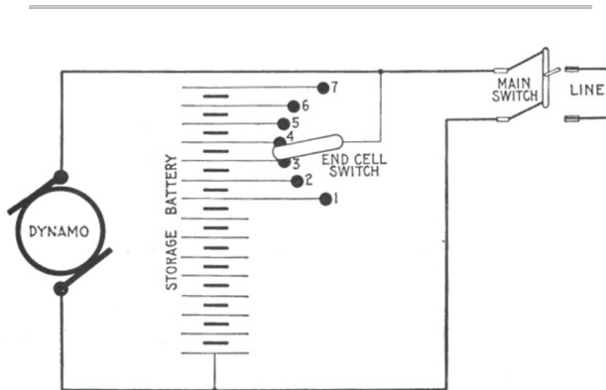
FIG. 1,188.—End cell switch control for storage battery; connections showing main line open when the battery is being charged.
