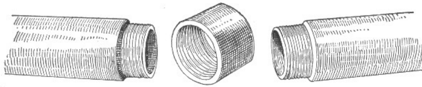
FIG. 986.—Screw joint type of fibre conduit. This method of connection will form a tight line and is suitable for running under the lawns of private houses and parks, under the streets of towns and villages, and in other places where the cost of building electric subways is prohibitive.
