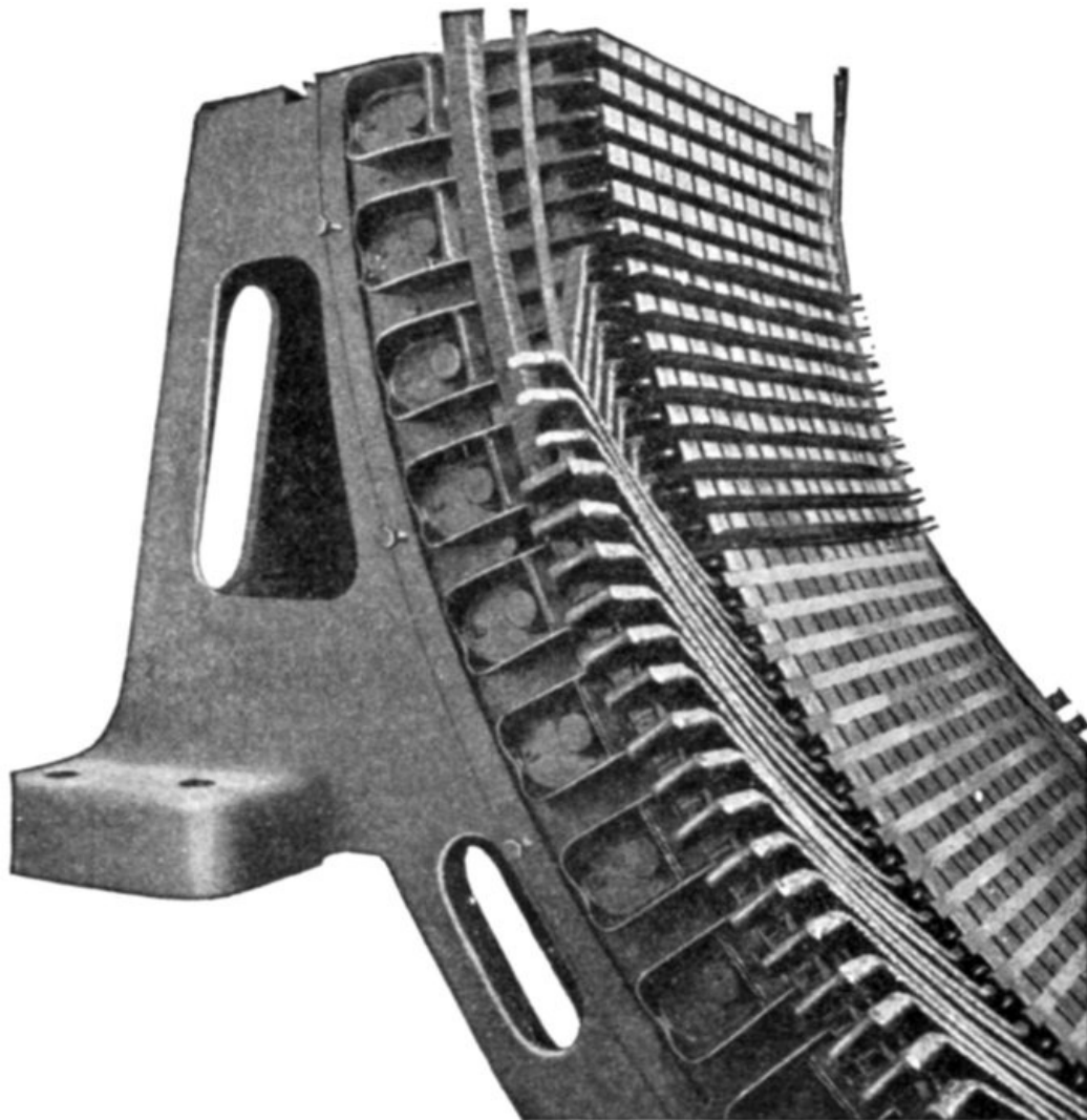
FIG. 1,484.—Section of General Electric stationary armature showing method of assembling the coils. These are form wound and are held in the slots by suitable wedges, the open slot construction permitting the use of form wound coils that can be easily removed and replaced in case of damage. Where heavy windings project beyond the laminations, an additional support is provided by means of an insulated metal ring, to which the outer ends of the coils are fastened; the coils are thereby protected from mechanical displacement, or distortion due to the magnetic disturbances caused by violent fluctuations of the load or short circuits. The figure shows a section of a supporting ring of this type and indicates the method of connecting the coils to it. In order to admit of the prompt replacement of damaged coils, sufficient space is usually provided between the alternator bearings to allow ample movement of the armature to permit of ready access to both armature and field coils. Where space necessitates the use of a short shaft, access to the windings may be had by disconnecting some of the coils and lifting the upper half of the armature.
