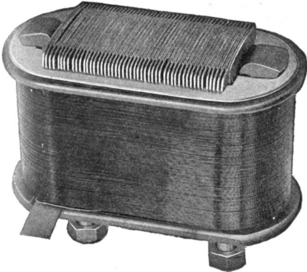
FIG. 1,468.—General Electric field coil showing another method of winding. The field coils on the larger machines consist of a single strip of flat copper, wound on edge as shown, so that the surface of every turn is exposed to the air for cooling. The flat sides of the copper strip rest against each other and the entire coil forms a structure of great solidity which can be easily removed for inspection and repair.
