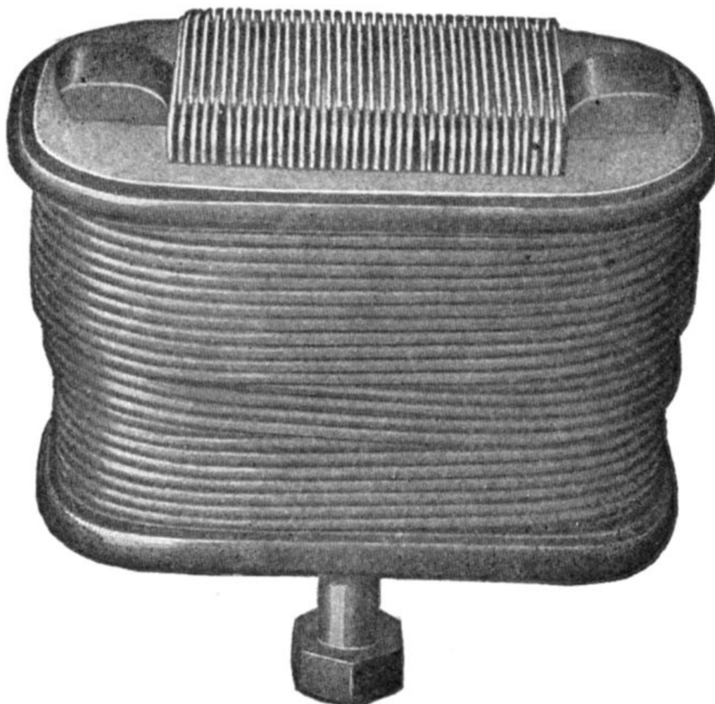
FIG. 1,467.—General Electric field coil, showing one method of winding. In the smaller machines the wire is wound on spools which are slipped over the pole pieces, which are built of sheet iron, spreading at the pole face so as to secure not only a wide polar arc for the proper distribution of the magnetic flux, but also to hold the field windings in place.
