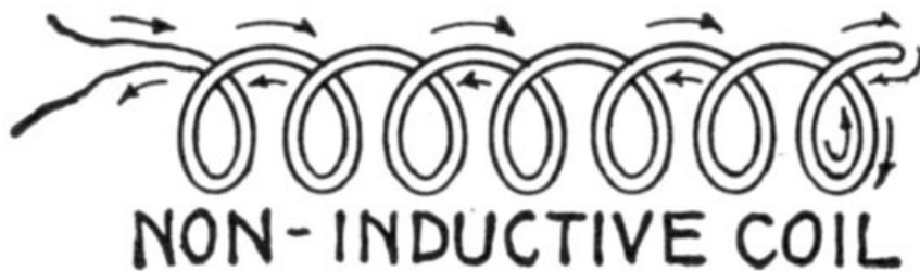
FIGS. 1,268 TO 1,270.—Various coils. The inductance effect, though perceptible in an air core coil, fig. 1,268, may be greatly intensified by inserting a core made of numerous pieces of iron wire, as in fig. 1,269. Fig. 1,270 shows a non-inductive coil. When wound in this manner, a coil will have little or no inductance because each half of the coil neutralizes the magnetic effect of the other. This coil, though non-inductive, will have "capacity." It would be useless for solenoids or electromagnets, as it would have no magnetic field.
