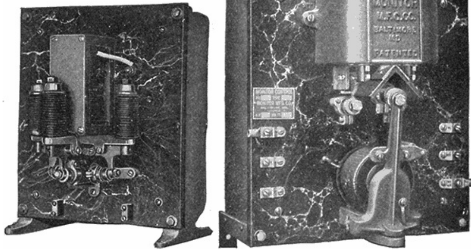
FIG. 749.--Monitor starter giving automatic start with knife switch control; designed for use with printing presses. It consists of a set of solenoids connected in series and so interoperating as to cut resistance out of the armature circuit of the motor as the apparatus it is driving comes up to speed. This type is for small motors or where no need arises for speed regulation; there is, therefore, no adjustment of speed possible aside from an actual change in motor conditions. At full speed the motor is directly across the main supply line.
