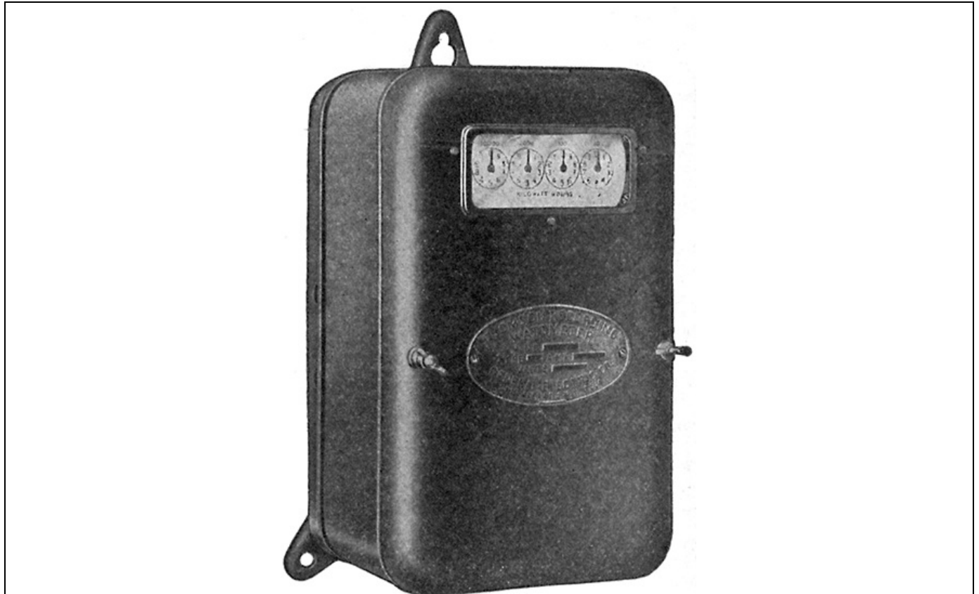
FIG. 653.--Thompson watt hour meter (type C-6). This form is furnished with side connections, the line wires entering at the left and the load wires at the right. Both sides of the system are carried through the meter in all sizes up to and including the 50 ampere size. In meters of larger ampere capacities, a voltage tap is used.
