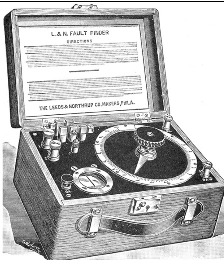
FIG. 587.--Leeds and Northrup fault finder. A lineman's instrument for the location of faults, crosses, grounds, and opens in telephone and telegraph circuits, and for the measurement of conductor and insulation resistance.
