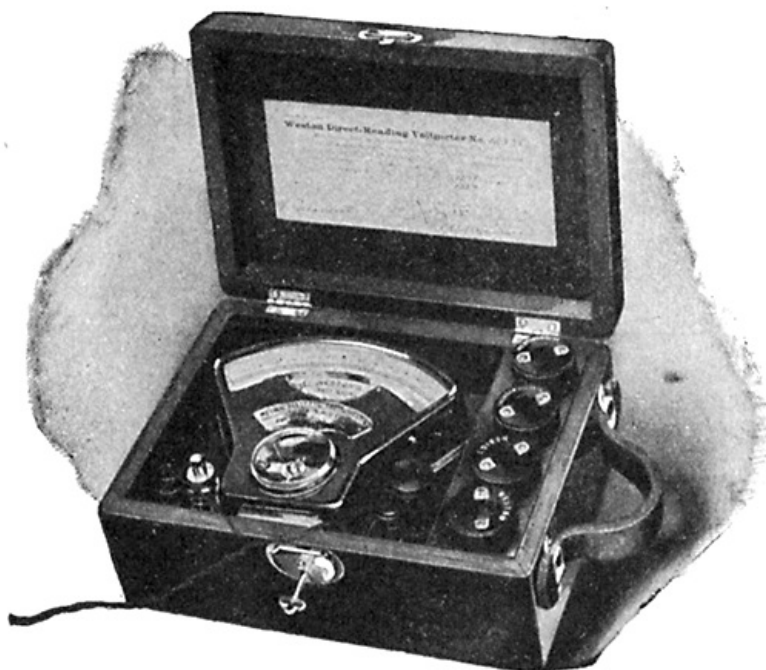
FIG. 632.--Weston portable voltmeter, inspector's style. This instrument is provided with a reversing key. Instead of the regular binding posts, pins are used with which connections are made by means of contact cups attached to flexible cords. These contact cups are convenient in making connections, or in changing quickly from one range to the other, if the instrument have a double scale. Connections for the different ranges are made in precisely the same way as with the regular double scale voltmeters. For the upper scale values, the contact pin to the right and the front contact pin to the left being taken, and for the lower scale values, the left contact pin is changed to the rear contact pin.
