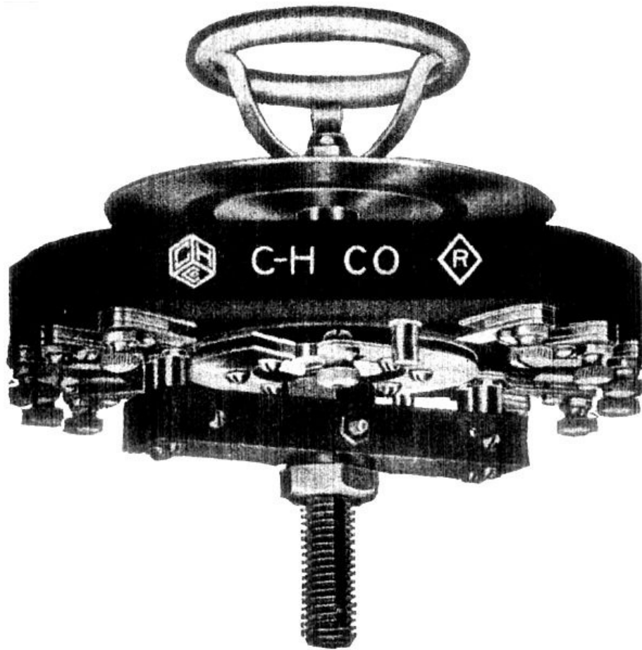
FIG. 2,669.—Crouse-Hinds radial ammeter switch, arranged for mounting directly on the switchboard. It is designed for use with external shunt ammeters of any make or capacity, and in connection with the required number of shunts, makes possible the taking of current readings of a corresponding number of circuits by means of one ammeter. The wiring diagram is shown in fig. 2,670 .
