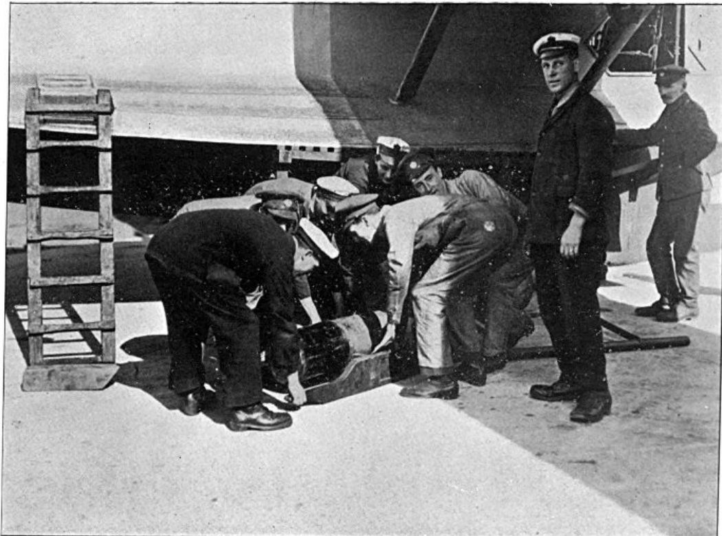
Lifting 230-lb. bomb into place.
