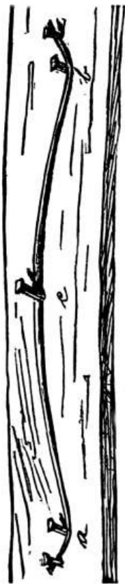
Fig. D. (A and B are six inches from the ends. The bow is bent slightly at C.)
