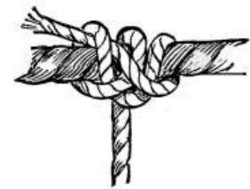
FIG. 25.—TO TIE A SHORT LINE, TO WHICH A HOOK IS ATTACHED, TO A LONGER OR GROUND LINE.
