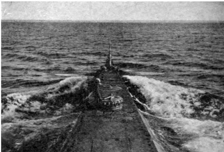
Same, preparing to submerge. Railing stowed away and bow-rudders extended.
