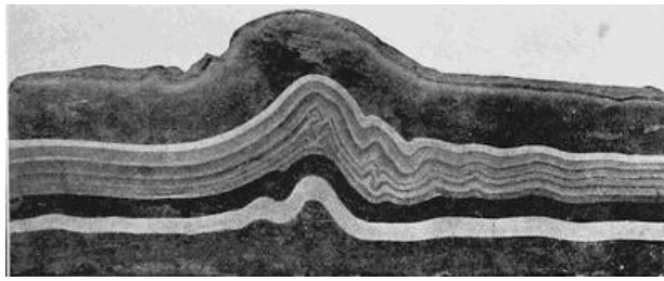
A. Layers compressed in experiments and showing the effect of a competent layer in the process of folding (after Willis).
