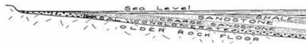
FIG. 18.—Diagram to show the order of the sediments laid down during a transgression of the sea.
