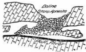
FIG. 197.—Cross section of the doline formed by inbreak of a cavern roof. The Stara Apnenka doline in Carinthia (after Martel).
