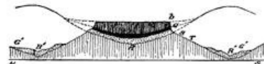
FIG. 108.—Diagram to show the manner of formation of mesas or table mountains by the outflow of lava in valleys and the subsequent more rapid erosion of the intervening ridges. R, earlier river valley; R'R', later valleys.
