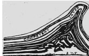
FIG. 153.—Result of experiment with layers of composition to illustrate the effect of relief of load upon rocks by arching of competent formation (after Willis).
