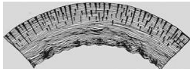
FIG. 26.—A bent stratum to illustrate tension upon the convex and compression upon the concave side (after Van Hise).
