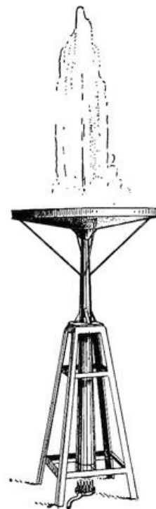
FIG. 203.—Apparatus for simulating geyser action in the lecture room (by courtesy of Professor B. W. Snow).
