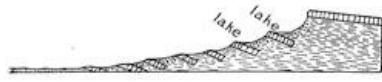
FIG. 449.—Lake basins produced by successive slides from the steep walls of a glaciated mountain valley (after Russell).
