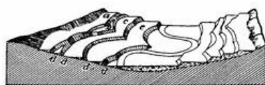
FIG. 172.—Schematic representation of a series of river terraces. a, b, c, e , successive terraces in order of age. d, d, d, d , terrace slopes formed of meander scars.
