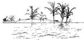
FIG. 75.—Settlement of a section of the shore at Port Royal, Jamaica, during the earthquake of January 14, 1907, adjacent to a similar but larger settlement of the near shore during the earthquake of 1692 (after a photograph by Brown).
