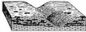
FIG. 191. —Diagram to show the relation of caverns in limestone to the river system of the district and to the "swallow holes" upon the surface.
