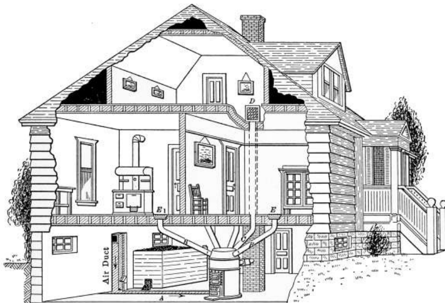
FIG. 48.—The hot-air furnace as it appears in the house.
