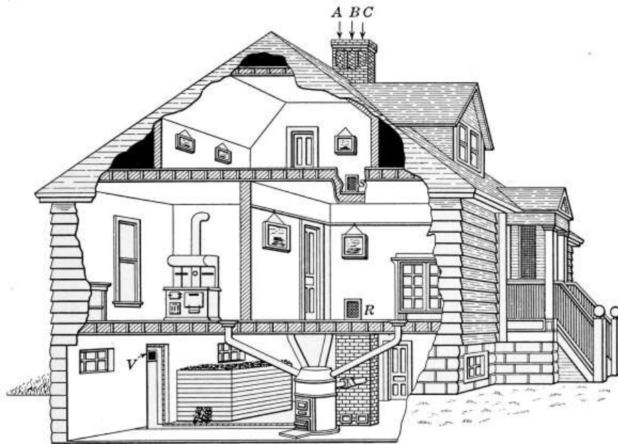
FIG. 163.—A chimney flue used as a ventilator.
