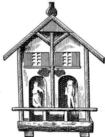
FIG. 161.—Swiss cottage "Barometer." This device is arranged to show the condition of atmospheric humidity by the movement of the images. It is not really a barometer.
