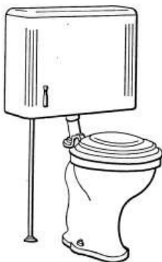
FIG. 108.—Siphon-jet closet with low-down tank.
