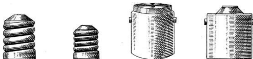
Candelabra screw base Miniature screw base Double-contact bayonet candelabra base Single-contact bayonet candelabra base
