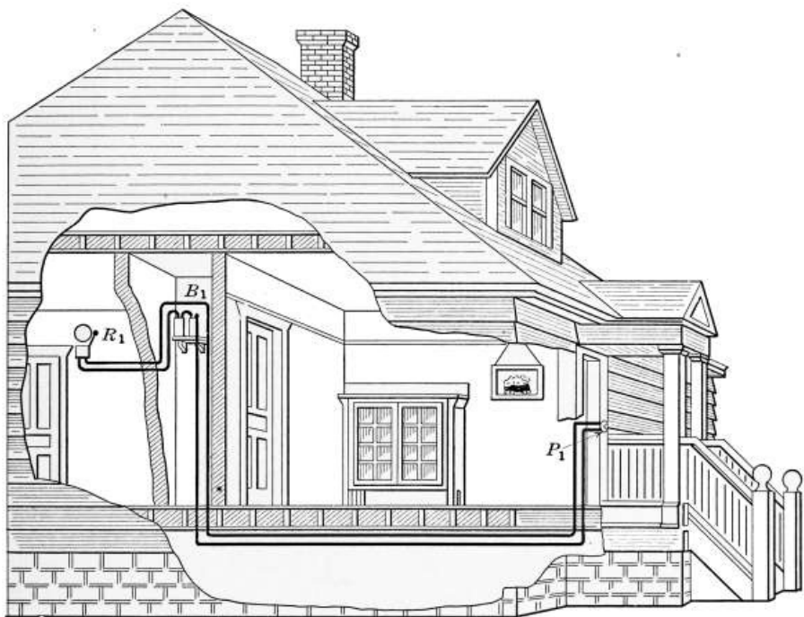
FIG. 239.—Example of an electric doorbell installation.
