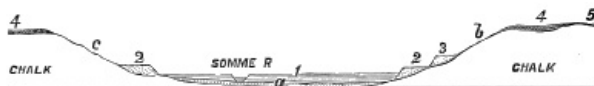
FIG. 77.—Section across valley of the Somme: 1, peat, twenty to thirty feet thick, resting on gravel, a ; 2, lower-level gravels, with elephant-bones and flint implements, covered with river-loam twenty to forty feet thick; 3, upper-level gravels, with similar fossils covered with loam, in all, thirty feet thick; 4, upland-loam, five to six feet thick; 5, Eocene-Tertiary.
