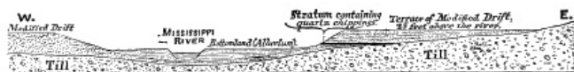
FIG. 73.—Section across the Mississippi Valley at Little Falls, Minnesota, showing the stratum in which chipped quartz fragments were found by Miss F. E. Babbitt, as described in the text (Upham).
