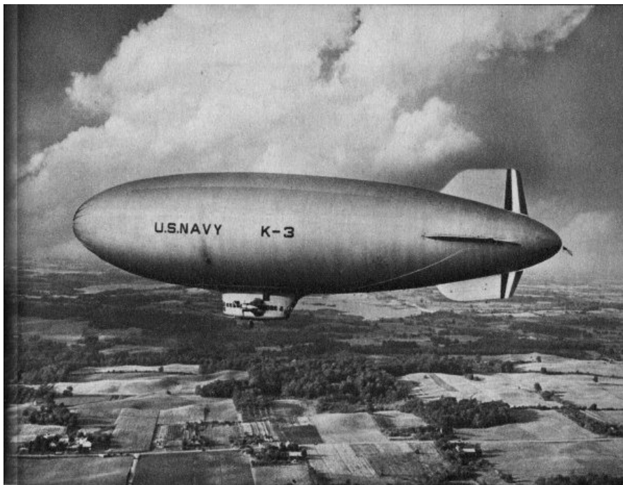
Helium-inflated, fast, long ranged, the modern K-type Navy patrol ship is a far cry from the primitive airships of World War I. They are armed with bombs and machine guns.
