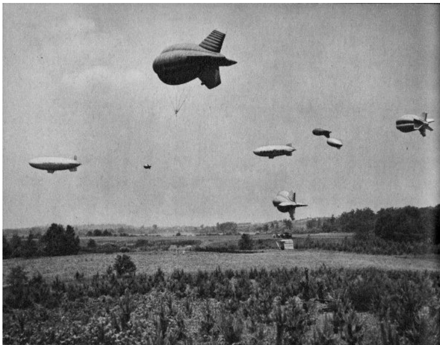
This Strata Sentinel will fly at 15,000 feet, twice the height of other barrage balloons. By that time the lobes will be completely filled out by expanding pressure of the lifting gas.
