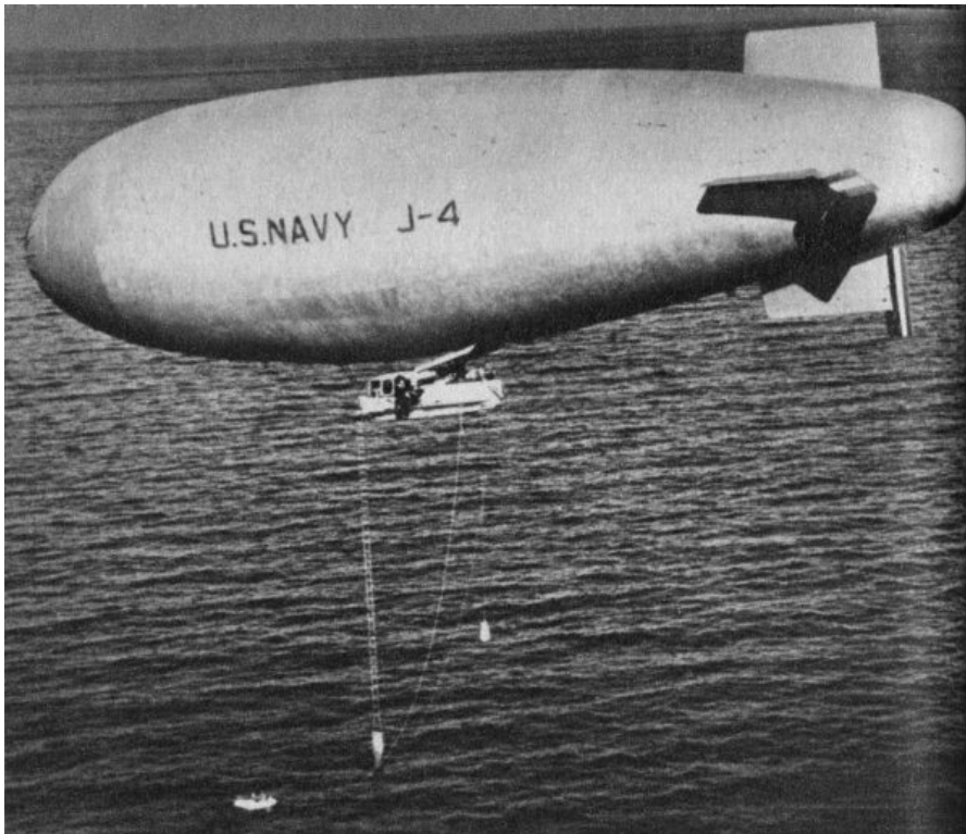
With a drogue or sea anchor to hold the airship steady, supplies or personnel may be taken aboard at sea. (U. S. Navy photo)
