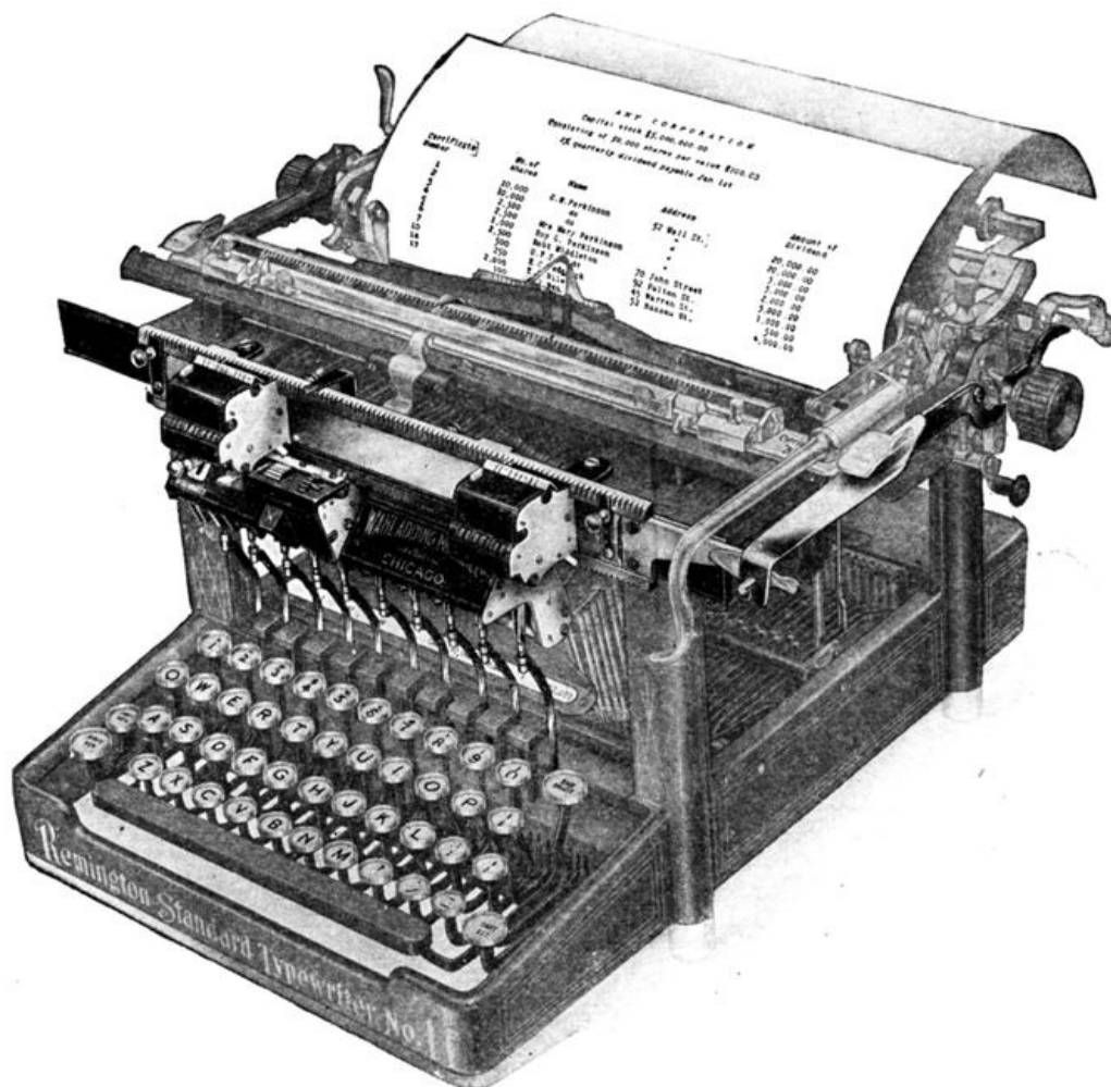
Fig. 29. Adding and Subtracting Machine Combined with Cylinder Billing Machine Remington Typewriter Co.
