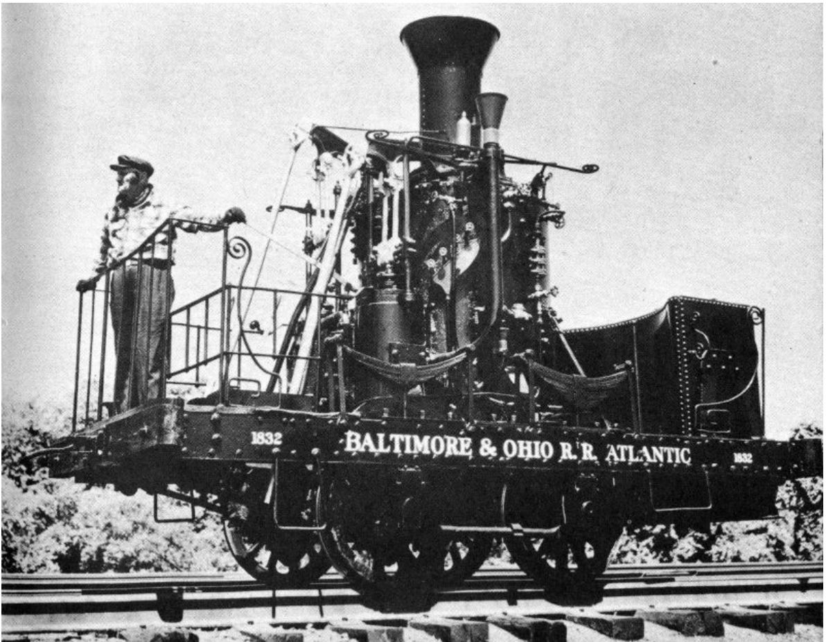
Figure 41.—Recent photo of so-called Atlantic . Note absence of side rod that originally connected the two axles.
