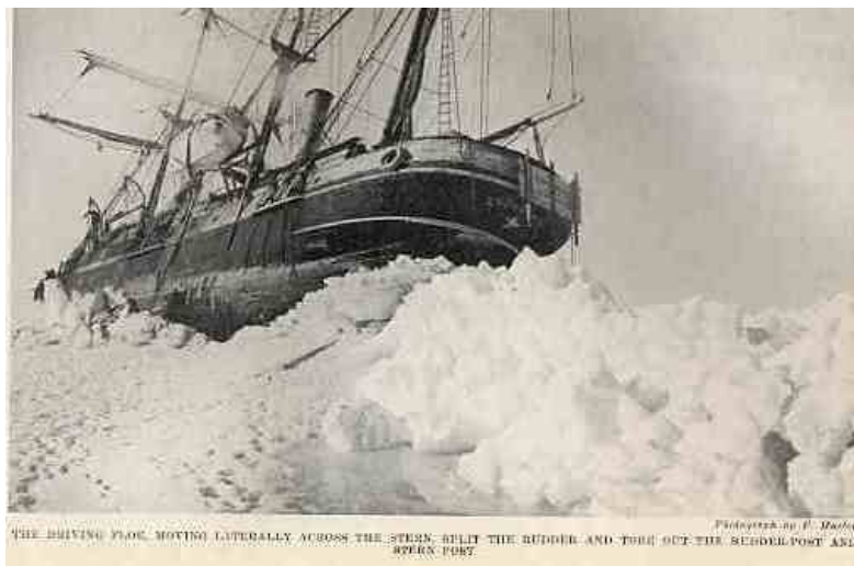
"The Driving Floe, moving laterally across the Stern, split the Rudder and tore out the Rudder-Post and Stern-Post"
