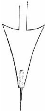
Fig. 381.— Manner of fastening Needle in Arrow-head.
