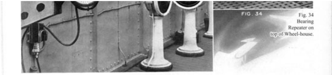
Fig. 33. Repeater at After Steering Station. Fig. 35. Repeater on Wing of Upper Bridge. Fig. 34. Bearing Repeater on top of Wheel-house.
