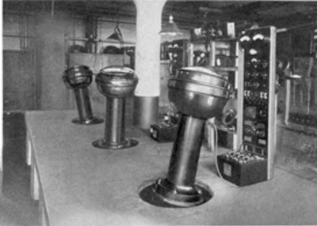
Master Compasses on Testing Machine which simulates the Roll, Pitch and Yaw of Ship at Sea.
