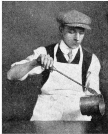
Fig. 22.—Soldering Can Externally
