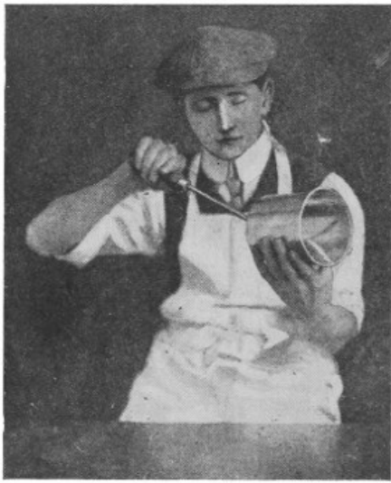
Fig. 20.—Soldering Internal Grooved Seam
