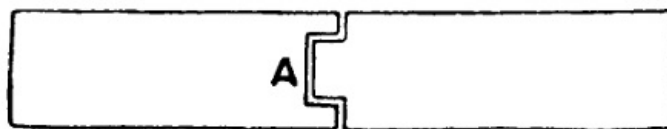
Fig. 45.—Aluminium Fitted Together for Soldering
