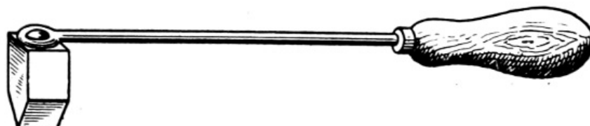
Fig. 6.—Hatchet Soldering Bit
