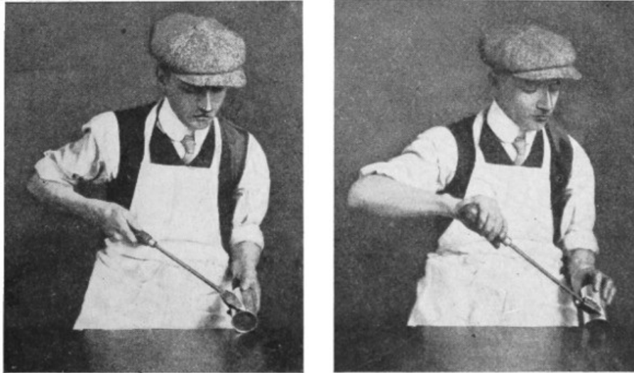
Figs. 18 and 19.—Incorrect and Correct Methods of Holding Bit
