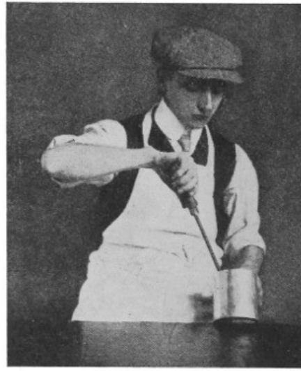
Fig. 21.—Soldering on Can Bottom Internally
