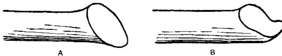
Fig. 66.—Scarfs for Iron and Steel
