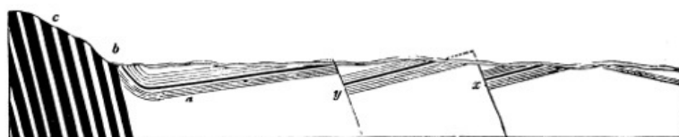
COAL BASIN OF CLACKMANNANSHIRE. a, b. Coal seams. c. Limestone strata. x, y. Slips.
