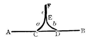
Answer.—The locomotive c backs a down and out toward A, then runs over toward B and backs b up on E F, then runs back toward B and goes over toward A, then runs up C E and draws b down on C E, then runs over toward A and gets car a, draws it over toward B and backs it up on D E. It can also be readily done by first backing a down on A C and drawing to and leaving it on C D.
