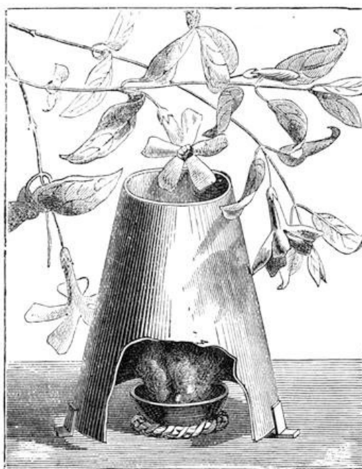
Fig. 317.—Discolouration of periwinkles by sulphuric acid.
