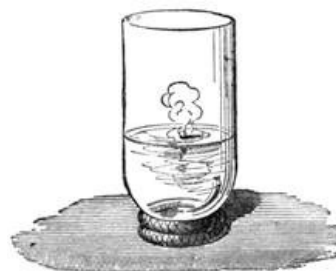
Fig. 305.—Combustion of sodium in water.
