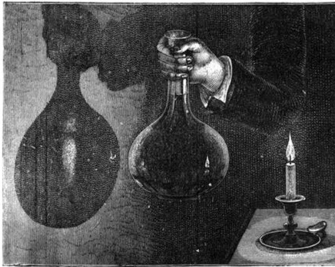
Fig. 90.—A water-bottle employed as a convergent lens.
