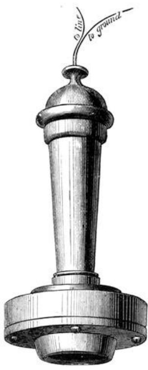
Fig. 192.—External appearance of Bell Telephone.
