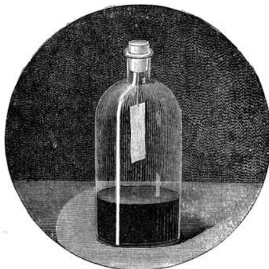
Fig. 316.—Gold-leaf exposed to the fumes of mercury.
