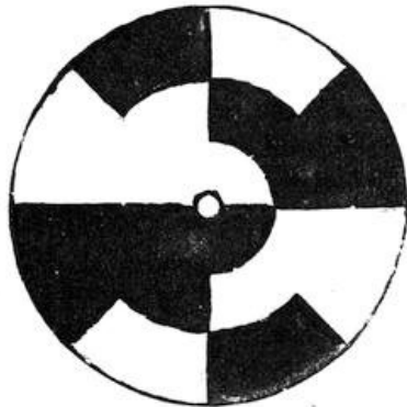
Fig. 105.—Disc which appears uniformly grey by reason of its rotation.
