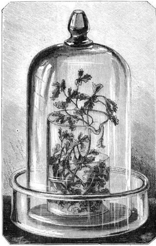
Fig. 10.—Arrangement of a microscopic aquarium for examining infusoria .
