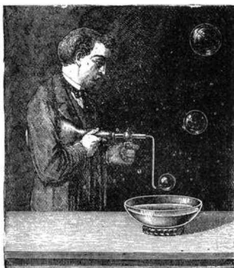
Fig. 341.—Blowing bubbles with hydrogen gas.
