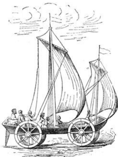
Fig. 491.—Sailing carriage of the 17th century, from a drawing of the period.
